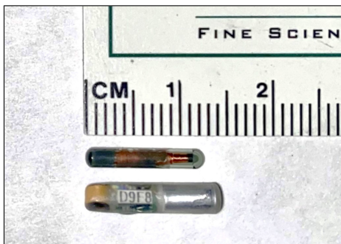
Figure 2-7. Juvenile Salmon Acoustic Telemetry System tag (model SS400; ATS, Inc., bottom tag) and passive integrated transponder (PIT) tag (top tag) that were surgically implanted into juvenile Puget Sound coho salmon in spring 2024.
