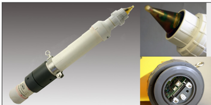
Figure 2-1. View of an autonomous receiver (left), a close-up of the hydrophone (top right), and a close-up of the internal (bottom right) components.
