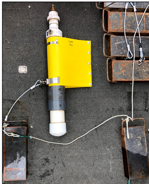
Figure 2-4. Autonomous receiver deployment rigging with a stabilizing fin (yellow piece affixed to the autonomous receiver).
