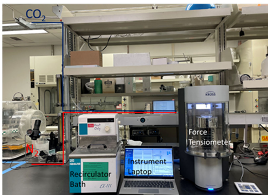
Fig. 4: Experimental setup including the KRÜSS K100C and its associated setup, a recirculatory bath, gas manifold, and instrument laptop. Surface tension measurement using the Wilhelmy plate method with the gas flow through the gas enclosure
