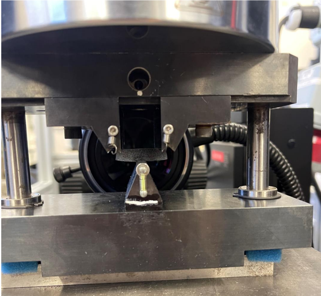
Figure 5. Short-beam shear testing setup for curved fiber-reinforced composites.
