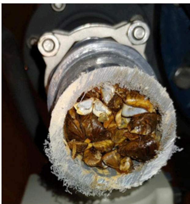
Figure 2: Zebra mussels clogging a pipe within a hydroelectric power plant in Gavins Point, South Dakota. (Photo by Michael Schnetzer, USACE).
