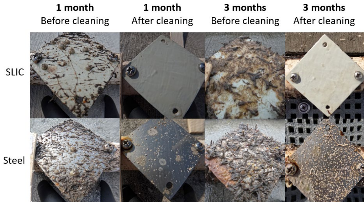
Figure 9: SLIC compared to bare steel 3 in x 3 in coupons after 1 month and 3 months of exposure to marine fouling in Miami, FL. Samples were photographed before and after they were cleaned with a common garden hose.
