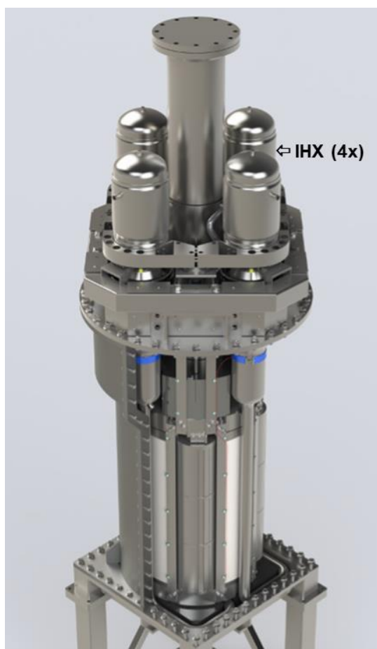
Figure 6. Schematic of the internal heat exchangers within the MARVEL Microreactor (Laboratory, 2022)
