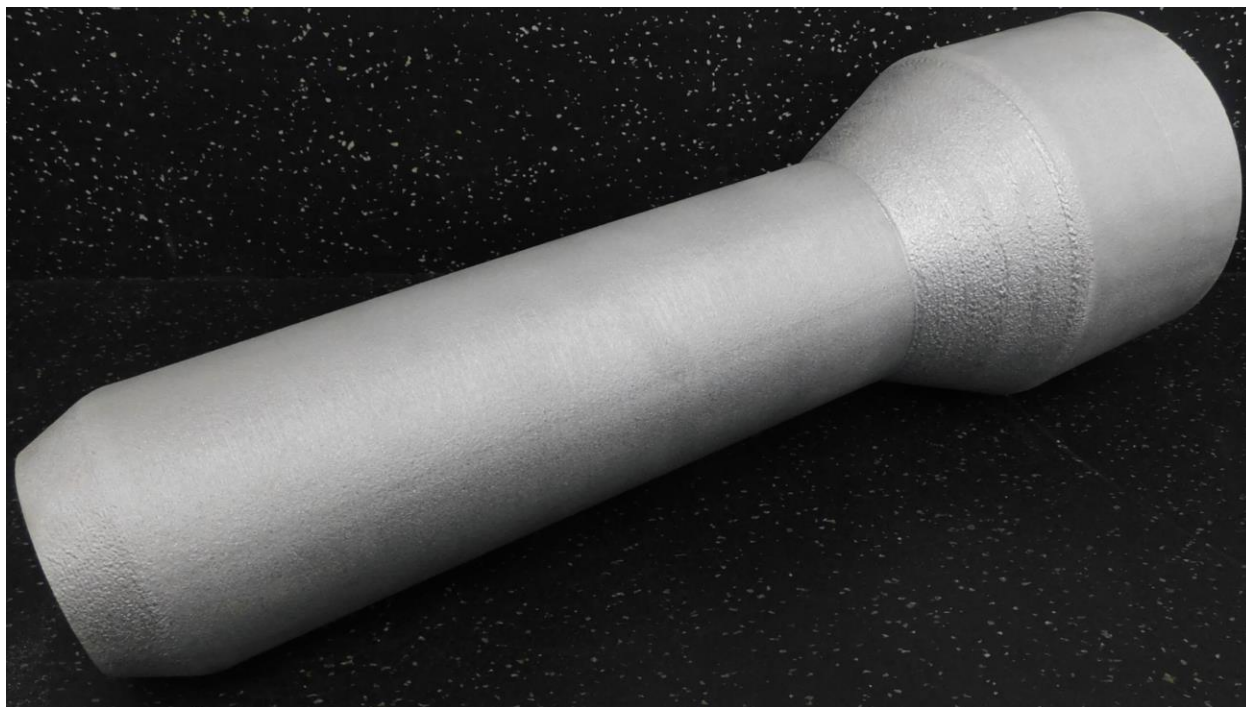
Figure 50. Completed DED liner removed from the baseplate
