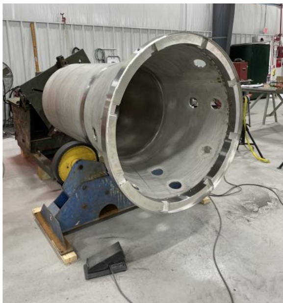
Figure 5. Example of guard vessel (Jackson, 2024)
