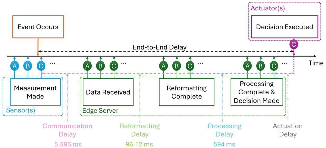
Figure 2-9 End-to-end delay composition with averaged measurements in the 5G-enabled protection example.
