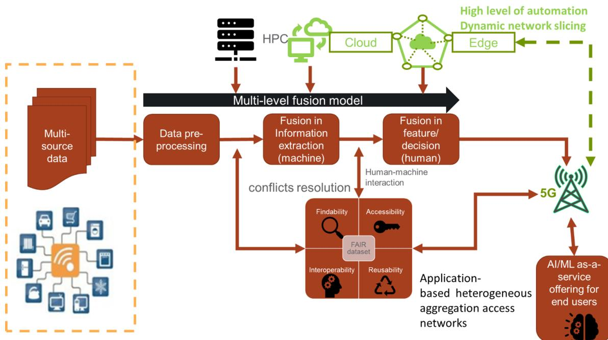
Figure 4-1 Data fusion framework integrated with various computing sources and 5G [48].
