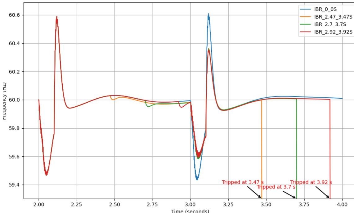
Figure 3-10: Comparison of inverter frequencies at node 806 (IBR 2) at the feeder 10 for four scenarios: no IBR tripping, and tripping with delays of 0.47 seconds, 0.7 seconds, and 0.92 seconds after fault 1 at 2.0 seconds and fault 2 at 3.0 seconds, with each fault lasting 0.1 seconds.
