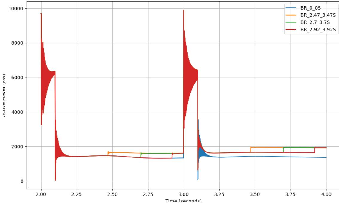
Figure 3-8: Comparison of active power at feeder 10 for four scenarios: no IBR tripping, and tripping with delays of 0.47 seconds, 0.7 seconds, and 0.92 seconds after fault 1 at 2.0 seconds and fault 2 at 3.0 seconds, with each fault lasting 0.1 seconds.
