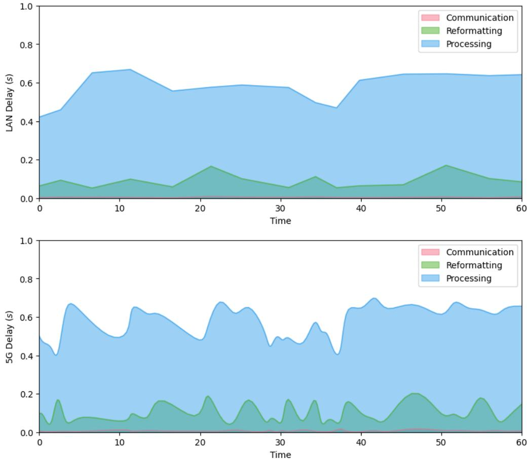
Figure 2-7: System performance illustration for the online grid edge computing with CNN model in LAN and 5G network configurations, respectively. The horizontal axis is the system operation timestamp at real-time and the vertical axis is the stacked delay, consisting of communication, reformatting, and processing delays.
