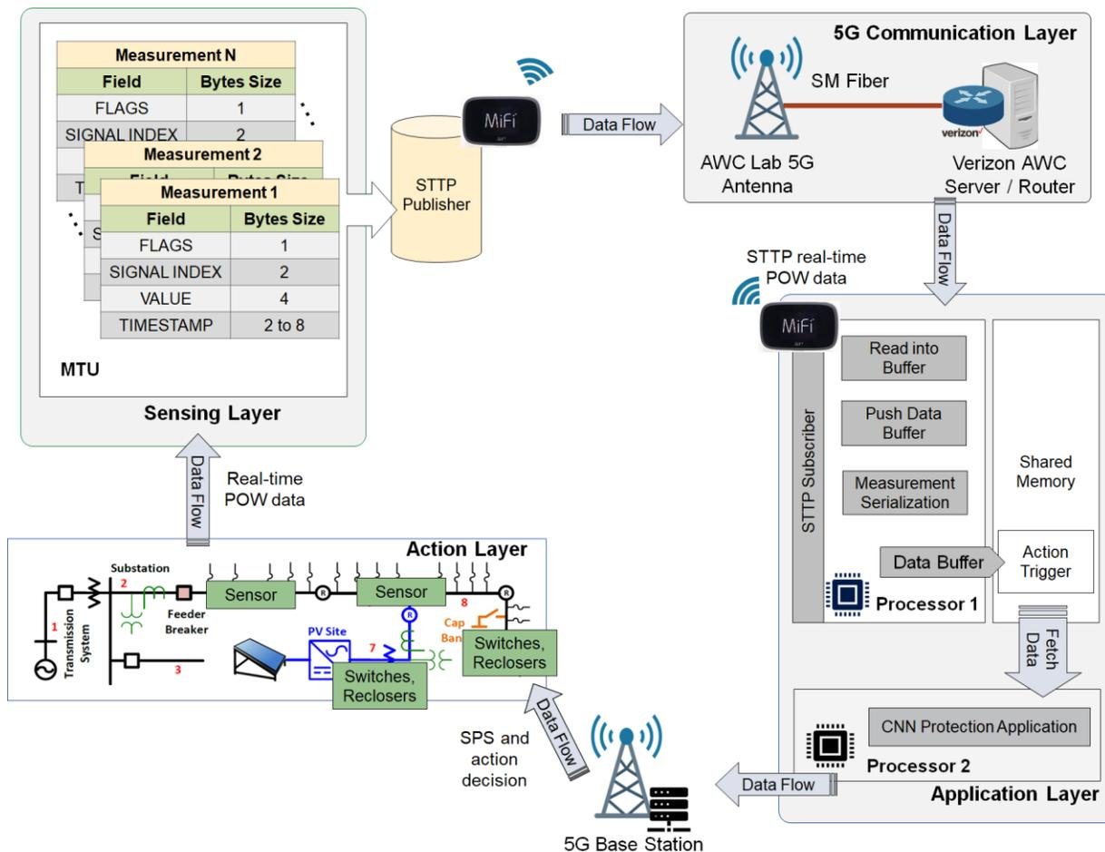
Figure 2-2. The data flow in the designed 5G-enabled grid protection framework.
