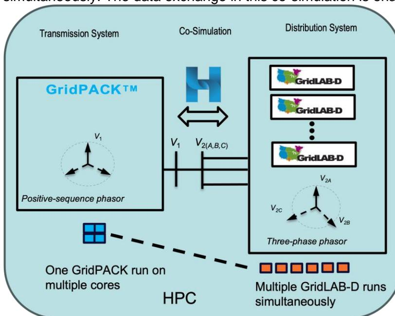
Figure 3-2 An illustration of power grid transmission and distribution co-simulation workflow using GridPACK, GridLAB-D, and HELICS.
