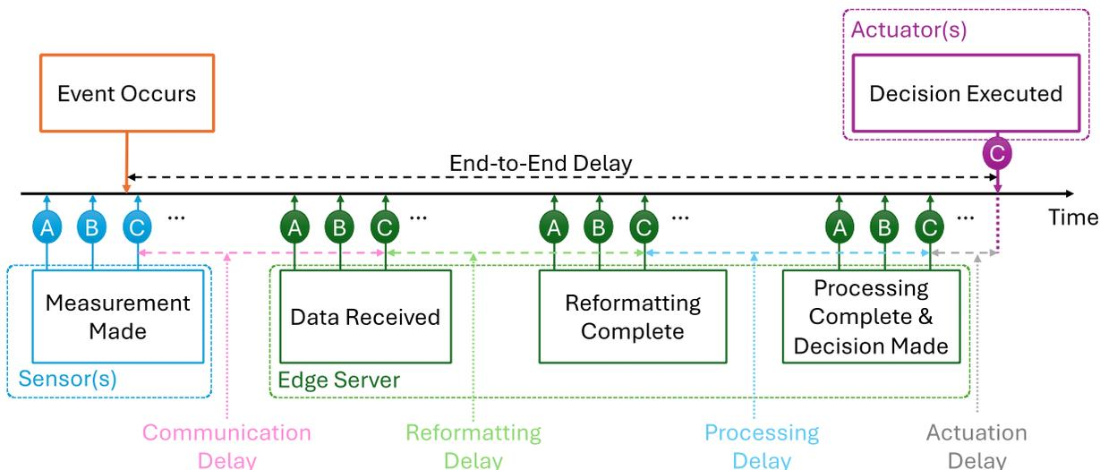
Figure 2-1 An illustration of power grid event monitoring and control/actuation process considering various types of latency/delay.
