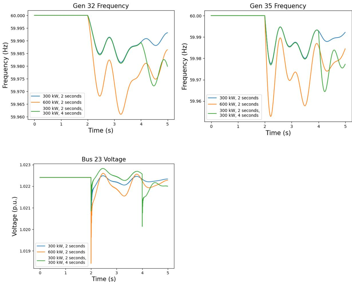
Figure 3-4 Frequency and voltage simulation results of two GFM IBRs tripping, each rated at 300 kW, using the example given in Figure 3-2 [41].
