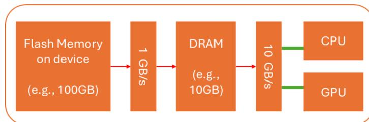
Figure 1-4 An illustration of different bandwidths among flash memory, DRAM, and CPU/GPU caches and registers within a single device.
