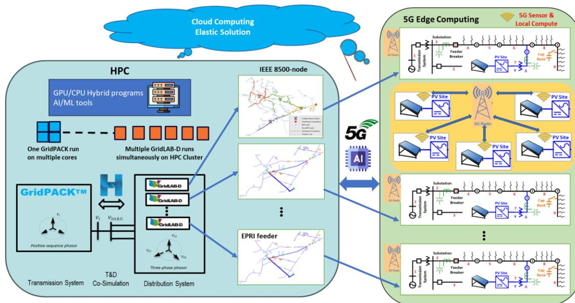
Figure 3-1 A detailed 5G-enabled power grid transmission, distribution, and communication co-simulation use case [40].
