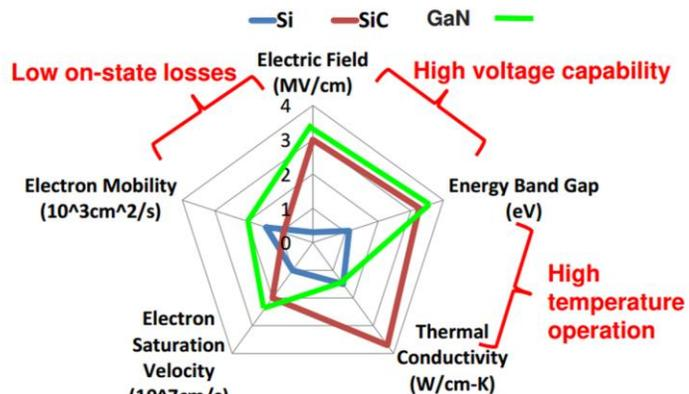
Figure 4-2 Performance comparison of semiconductors from power electronics perspective [53].
