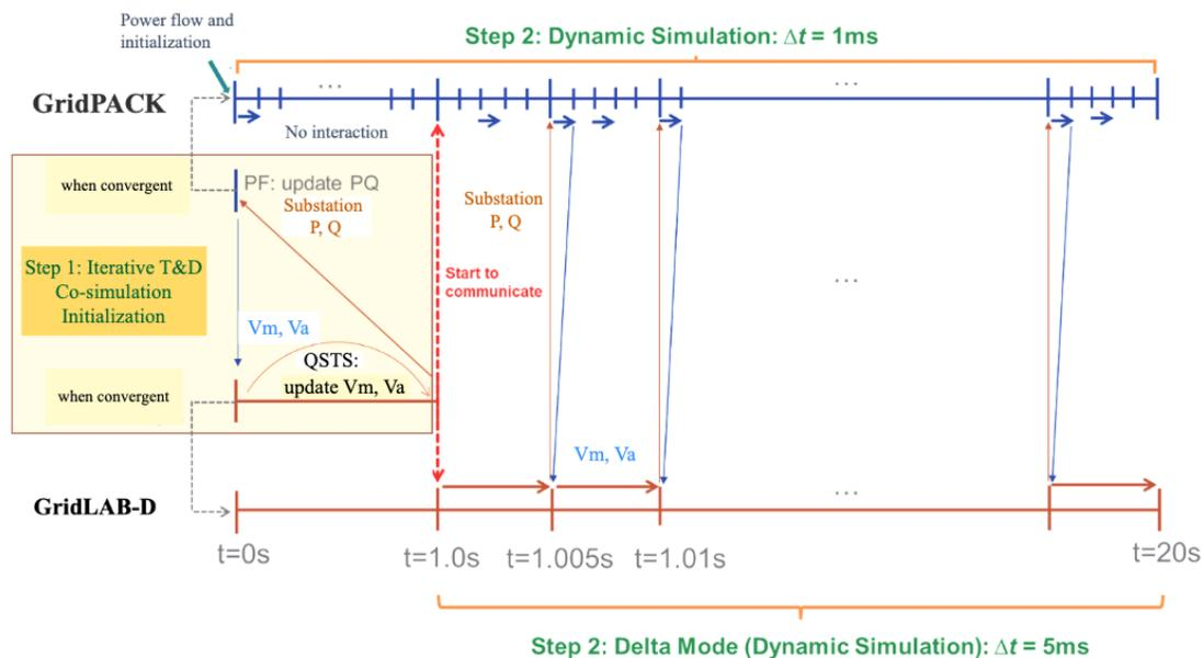
Figure 3-3: The co-simulation mechanism between GridPACK and GridLAB-D enabled by HELICS, where the time steps for GridPACK/HELICS/GridLAB-D are 1ms/5ms/5ms, respectively [41].
