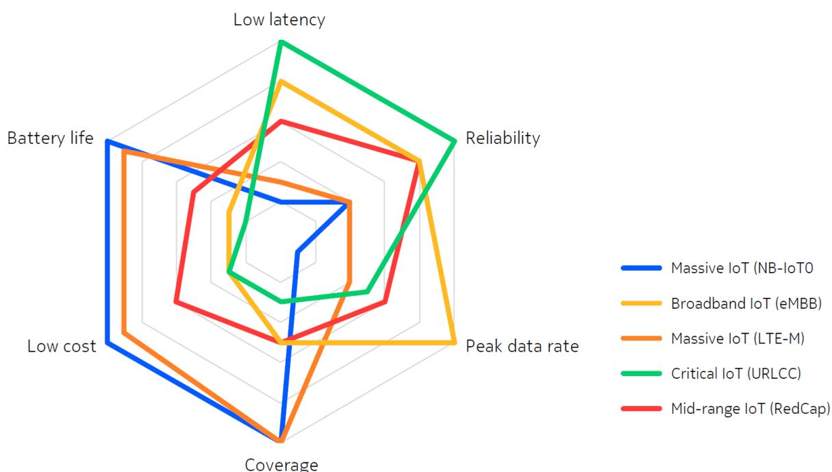
Figure 1-6 An illustration of 5G RedCap equipment capability and a group of IoT use cases mapping to 5G characteristics [35].
