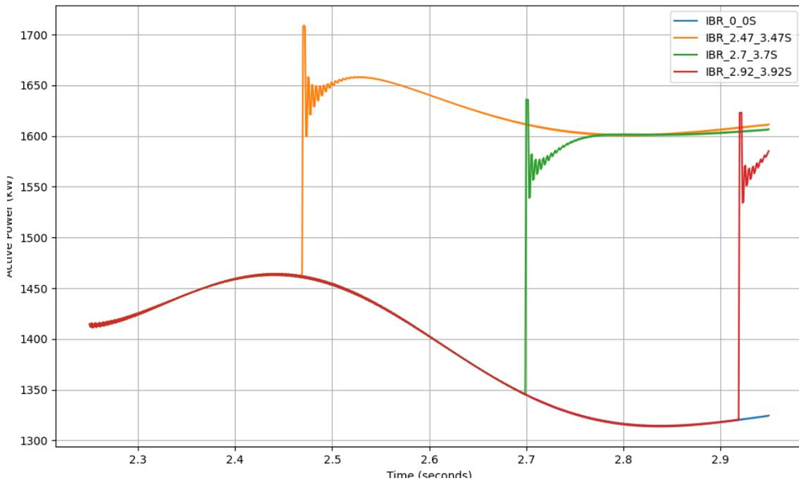
Figure 3-9: Comparison of active power at feeder 10 for four scenarios: no IBR tripping, and tripping with delays of 0.47 seconds, 0.7 seconds, and 0.92 seconds after fault 1 at 2.0 seconds and fault 2 at 3.0 seconds, with each fault lasting 0.1 seconds, focusing on four IBR tripping scenarios during 2.25 seconds to 2.95 seconds.
