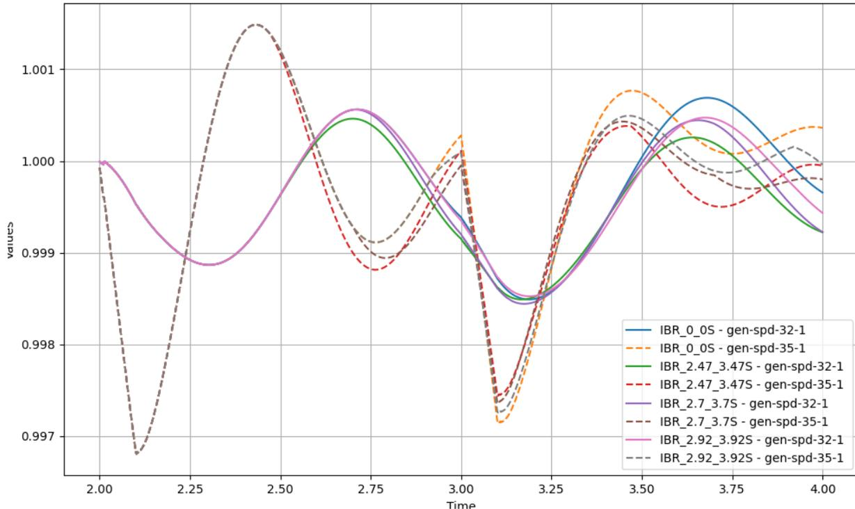
Figure 3-7: Comparison of generator frequencies at generator 32 and generator 35 for four scenarios: no IBR tripping, and tripping with delays of 0.47 seconds, 0.7 seconds, and 0.92 seconds after fault 1 at 2.0 seconds and fault 2 at 3.0 seconds, with each fault lasting 0.1 seconds.
