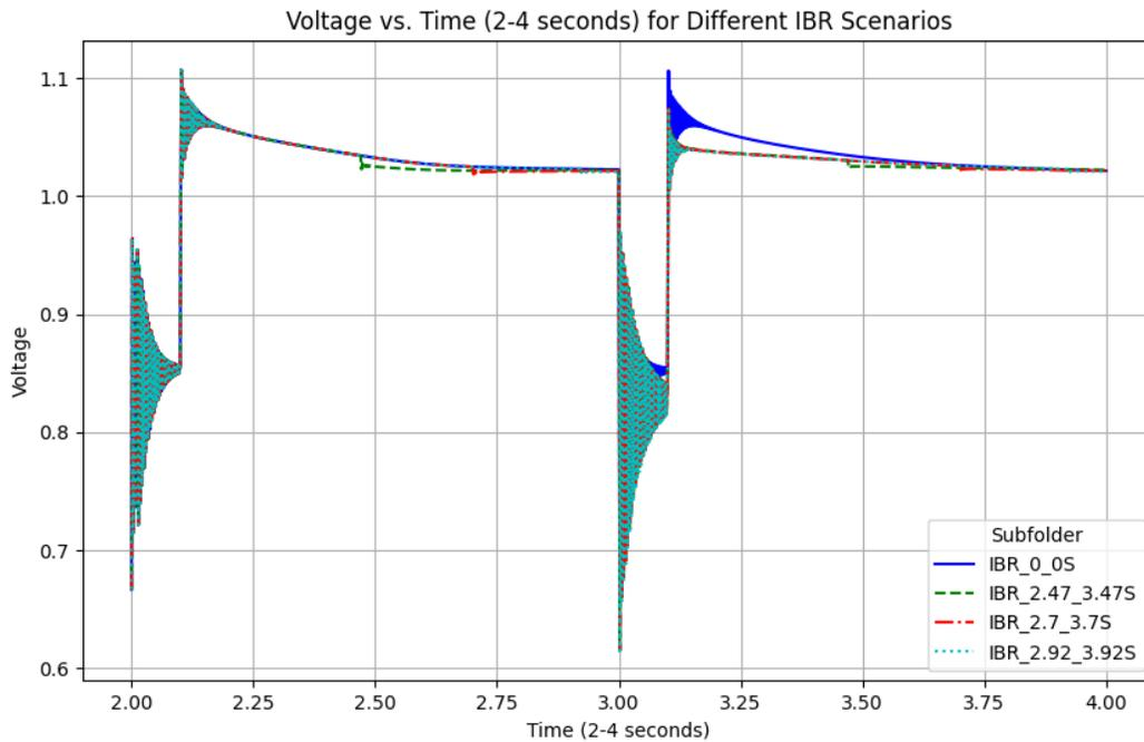
Figure 3-6: Comparison of voltage magnitudes at bus 23 for four scenarios: no IBR tripping, and tripping with delays of 0.47 seconds, 0.7 seconds, and 0.92 seconds after fault 1 at 2.0 seconds and fault 2 at 3.0 seconds, with each fault lasting 0.1 seconds. The figure is zoomed in between 2.0 and 4.0 seconds.
