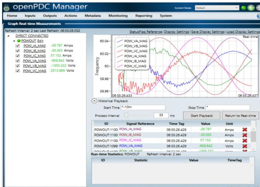
Figure 2-5 Generate 10k sample/second POW streaming signals using OpenPDC.
