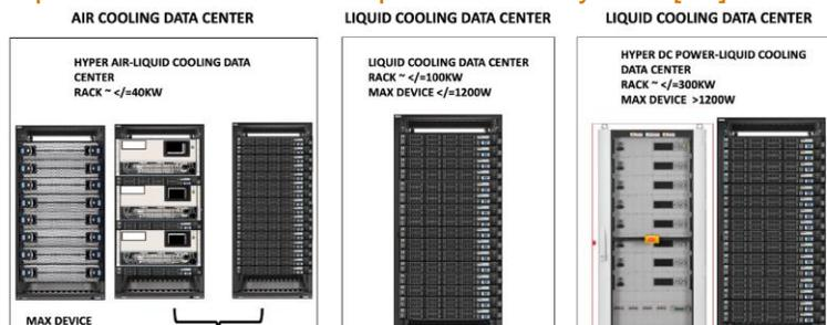
Figure 4-4 An illustration of different data center computing server rack and cooling solutions [54].
