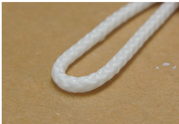
Figure 5: FlexiSLIC coated on nylon rope and bent. This illustrates the ability of the coating to flex as required for application on netting and ropes.
