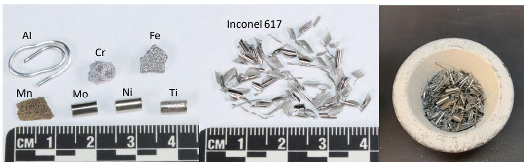
Figure 10. 4N to 5N elemental purity pure elements, left. IN617 filaments and chips, middle and alumina crucible with pure elements and IN617 ready for casting.
