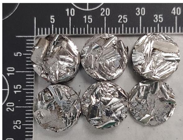
Figure 11. Pure metal components and Inconel 617 chips pressed into pellets.
