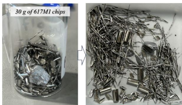
Figure 15. A mixture of Inconel 617 chips and pure metal alloying additions.
