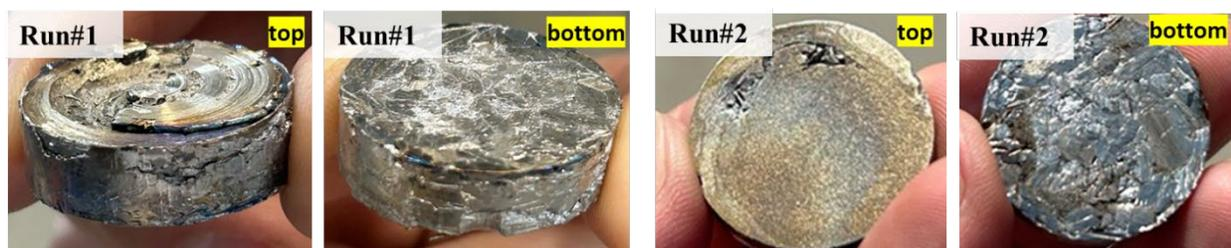
Figure 18. Top- and bottom view of consolidated and alloyed chips for Run #1 and #2.
