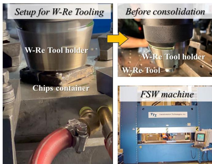
Figure 16. Friction consolidation and solid phase alloying setup.
