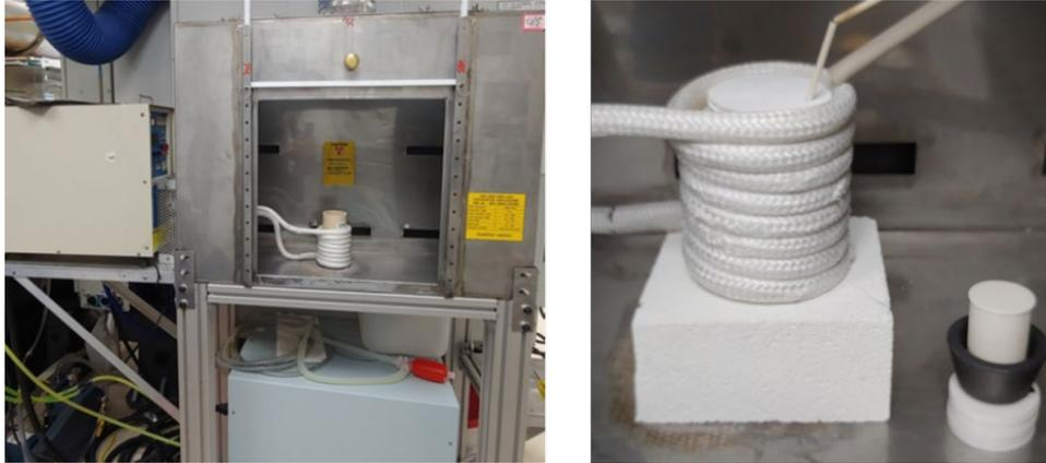
Figure 12. MTI 25 kW Induction furnace with induction coil, left, coil, insulation, and internal crucible setup used for alloying new metal compositions, right.
