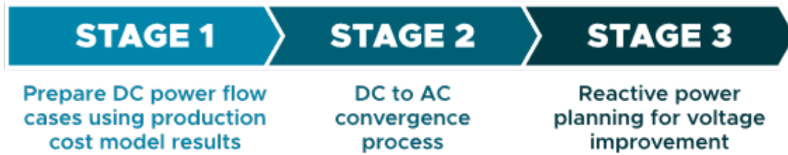
Figure 32. C-PAGE AC power flow three-stage convergence process.
