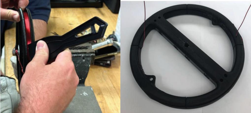
Figure 6. Left shows the winding process of the receiver coil former using AWG18 enameled copper wire. Care had to be taken to pack the turns in carefully so that wires from adjacent layers didn't come close to one another. Right shows the finished receiver coil. The coil has an inductance of 2.67 millihenries, a DC resistance of 1.09 $\Omega$ , and a self-resonance of 298.5 kHz.
