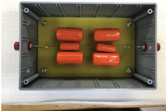
Figure 12. Photo of the capacitor box used to resonate the Tx coil. This consists of three parallel banks of caps, each consisting of a series string of two. Two of these strings comprise 220-nF caps, while the smaller central one comprises 47-nF caps. This gives a total capacitance of 243.5 nF.
