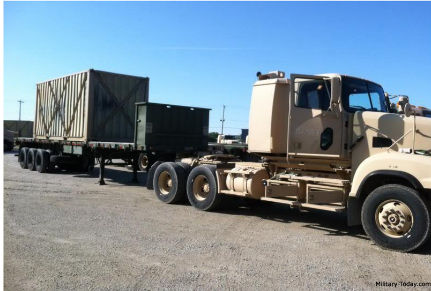
Figure 2.2. An Army M915A5 Tractor with a M872A4 Semi-Trailer Carrying a 20 ft ISO Container 4
