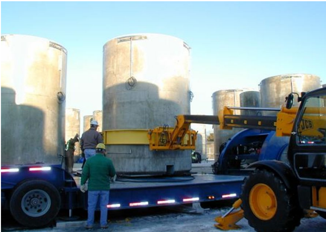
Figure 2-29: NAC VCC Movement from HHT to ISFSI Pad on Air Pads and Engaged to JCB Telescopic Handler
