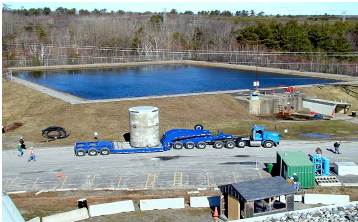
Figure 2-25: Loaded VCC on HHT
