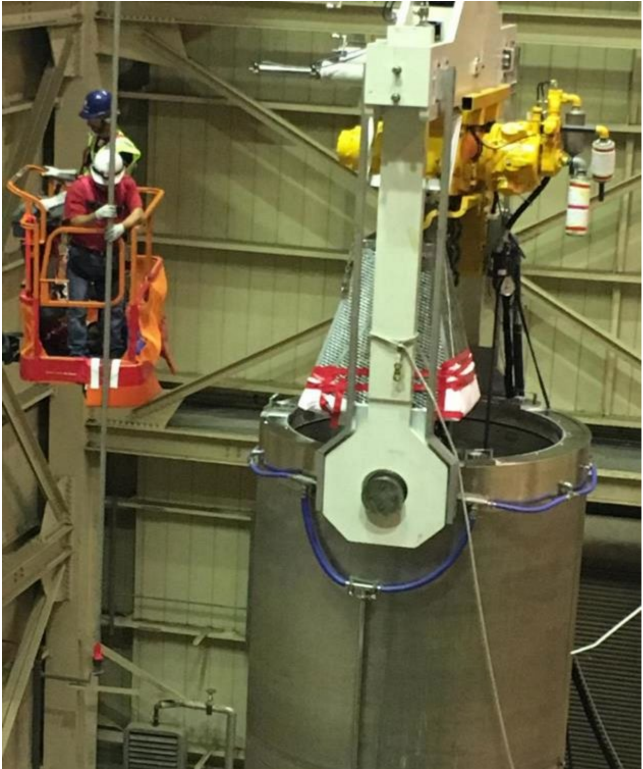
Figure 2-33: MAGNASTOR Transfer Cask [19] Engaged to Secure-Lift Yoke
