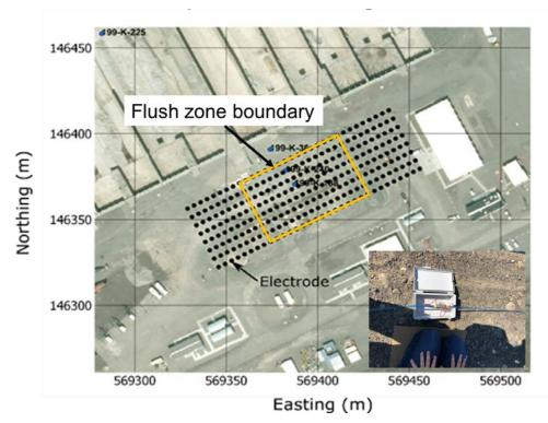
Figure 3. Location of surface ERT electrode lines (black dots) installed over the soil flushing zone. The lateral extent of the array, which impacts imaging depth, was limited by the building foundation located at the eastern margin of the array.
