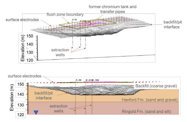
Figure 4. (top) Oblique view of the boundary between the pit backfill and the Hanford formation. (bottom) Cross-section showing the approximate position of the water table (blue inverted triangle), the Ringold Formation, the Hanford-Ringold formation contact, and the contact between the Hanford formation and pit backfill.
