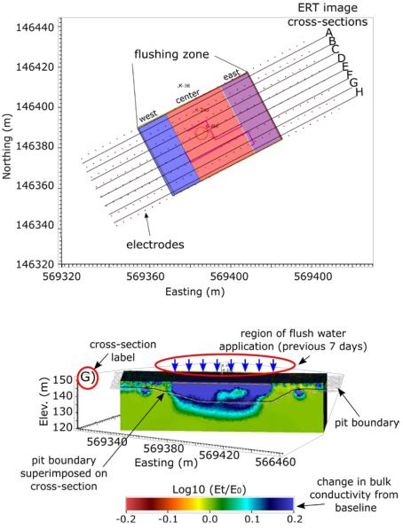
Figure 8. Locations of cross-sections used to present ERT imaging results.
