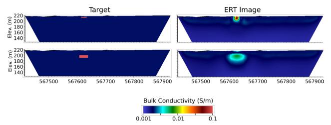
Figure A.2. Synthetic imaging example demonstrating the effects of limited resolution.
