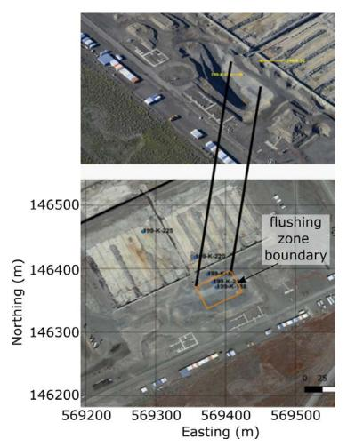
Figure 2. (top) Aerial view of the excavation pit constructed to removed Cr(VI)-contaminated sediments from the vadose zone. (bottom) Aerial of the soil flushing zone super-imposed on the backfilled excavation pit.
