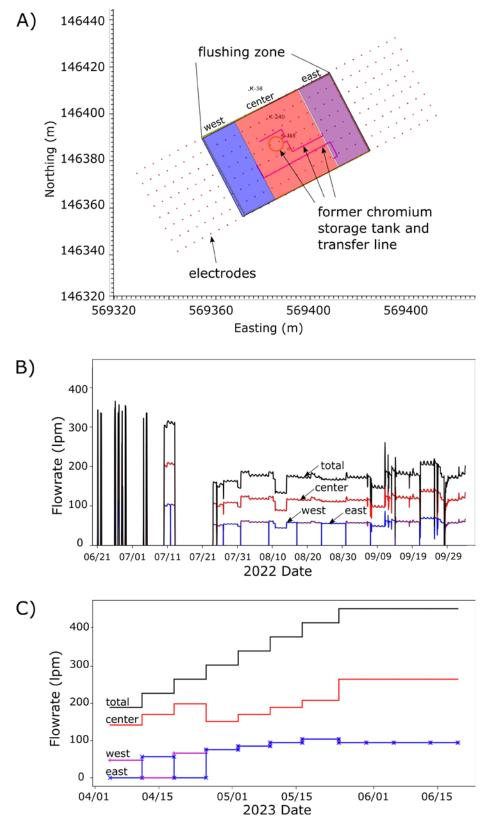
Figure 5. A) Flush water application zones. B) 2022 total and zonal flush water application rates. C) Nominal 2023 total and zonal flush water applications rates.
