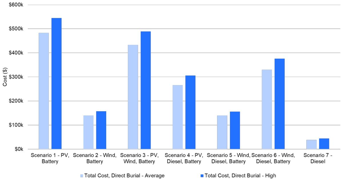
Figure 8. Cost summary for the installation of new distribution cable, 24/7 operations & electric landfill equipment.
