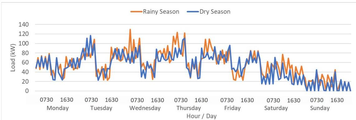
Figure 5. Estimated typical weekly Marpi Landfill load profile with electric equipment charging.
