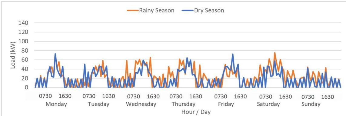
Figure 2. Estimated typical weekly Marpi Landfill load profile with 24/7 operations.
