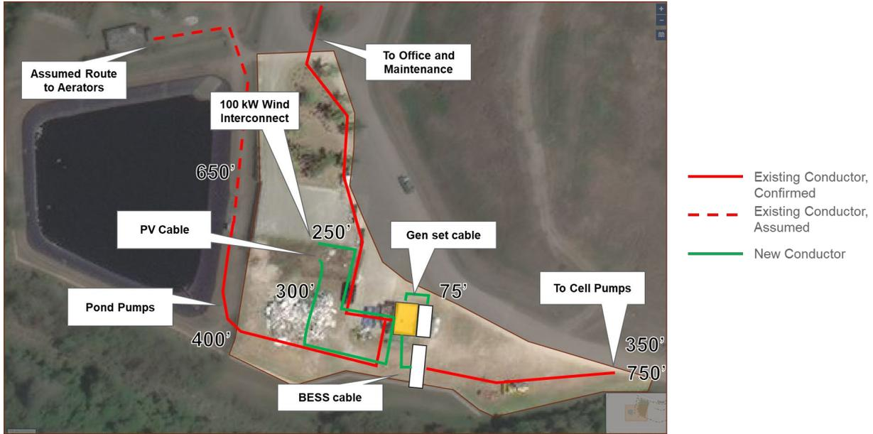
Figure 6. Overview of existing and new electric distribution cable.
