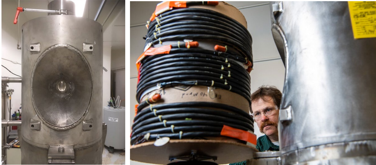
Figure 1. Front and side views of the gamma-ray irradiator in the PNNL High Exposure Facility. Shown is the mandrel assembly on a spinning 2-rpm turntable in position for long term exposure utilizing the upper 70° port.
