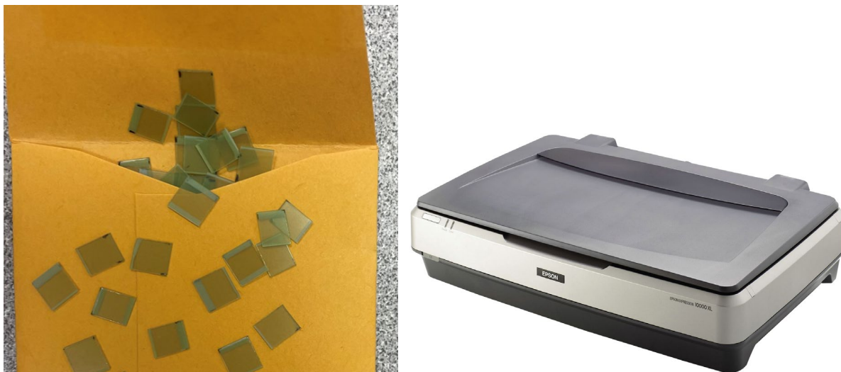
Figure 4. Samples of the MDV3 radiochromic film (left), and the EPSON model 10000XL flatbed scanner used to analyze the irradiated film.
