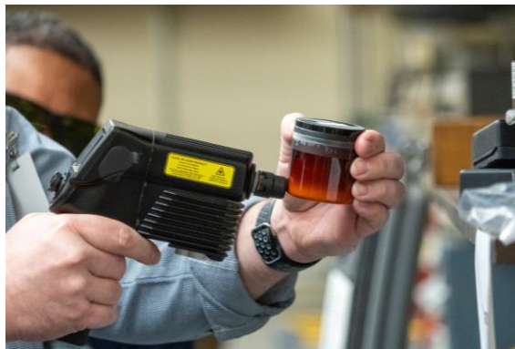
Figure 4-40 Chemring PGR-1064 being used to sample through an amber container
