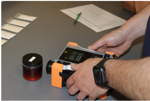
Figure 4-14 Rigaku ResQ CQL collecting a sample through an amber container
