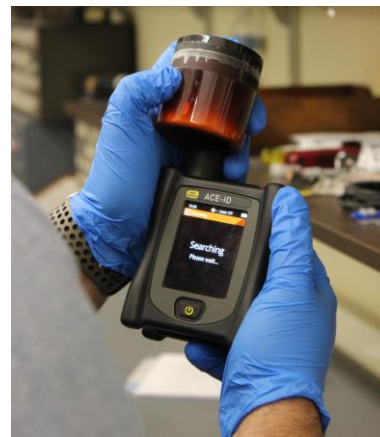
Figure 4-28 Evaluator sampling through an amber container using a Smiths Detection ACE-ID
