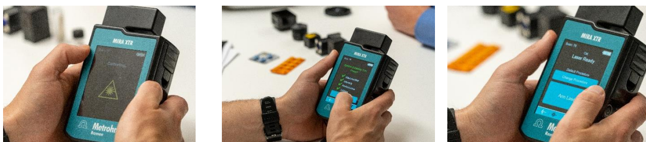
Figure 4-26 Metrohm Mira DS calibration phases
