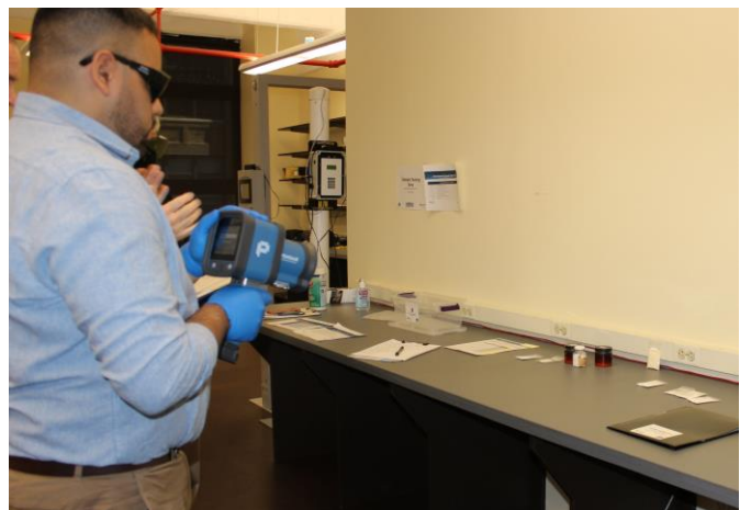
Figure 4-35 Pendar X10 being used for standoff measurement
