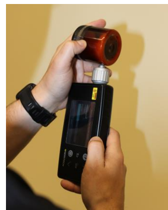
Figure 4-32 Sampling through an amber container using the Serstech Arx
