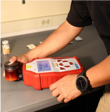
Figure 4-2 Evaluator scanning through an amber container
