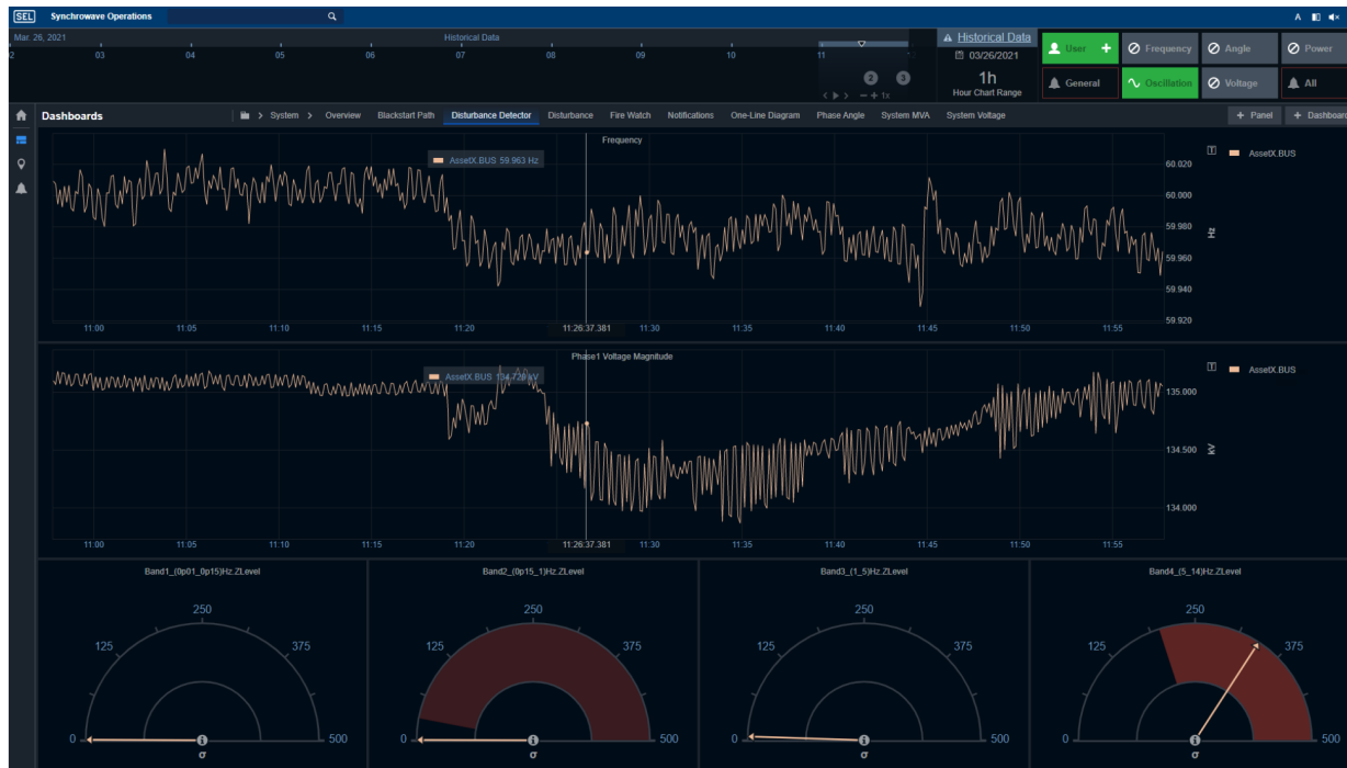
Figure 43. Disturbance detector dashboard in SEL’s Synchronwave showing a forced oscillation [Cassidoro, 2021]
