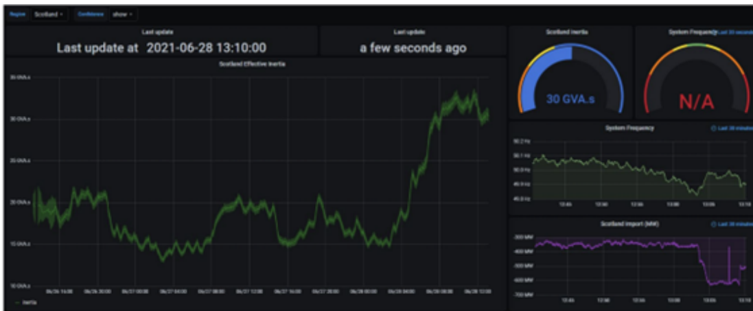
Figure 7. Dashboard at National Grid, UK with results from GE’s inertia monitoring tool. Source: National Grid [Dytham, 2021].
