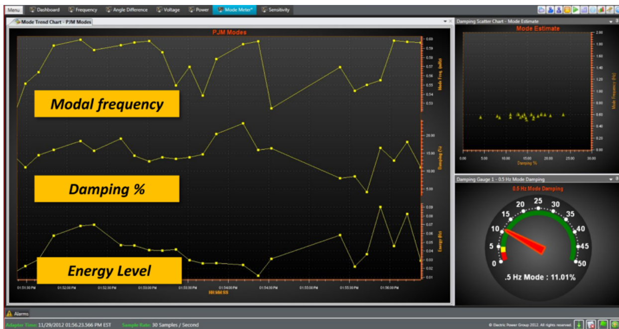
Figure 30. Mode monitoring display setup using EPG RTDMS, courtesy: EPG and ERCOT [EPG, 2014].
