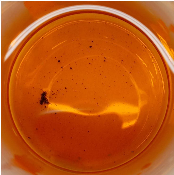
Figure 19. Photograph of 5 mM iodide solution in 0.5 M H_2SO_4 after completion of chronoamperometry experiment with addition of 0.1 M H_2O_2 .
