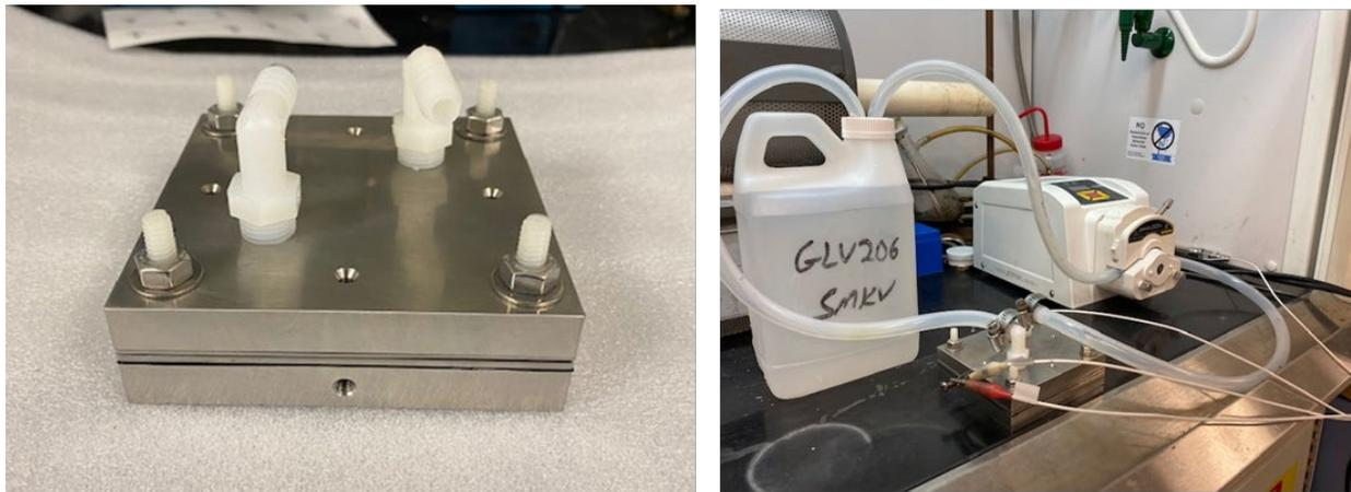
Fig. 4 Photo of the designed Li-extraction flow cell with a 2 in× 2 in working area (left) and the continuous operation of the Li-extraction flow cell (right).
