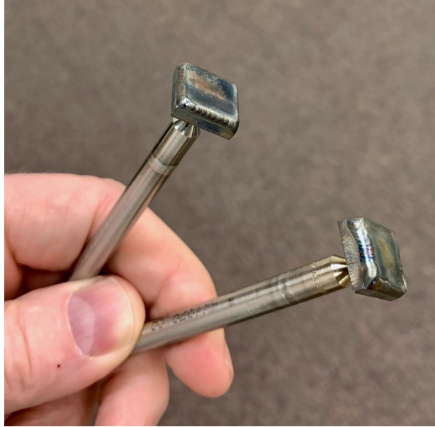
Figure 2.5. Test fixtures with pellets removed to test for H_2 permeation through the steel
