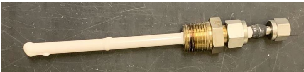
Figure 2.6. Test fixture made from three LiAlO_2 tubes bonded lengthwise
