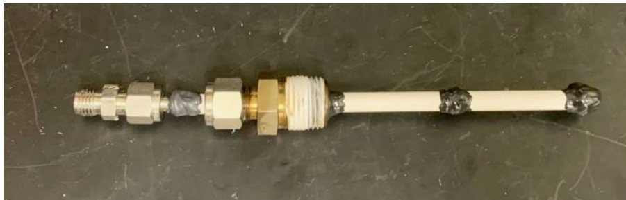
Figure 3.15. Unglazed 3-pellet test piece with epoxy covering joints and end-plug
