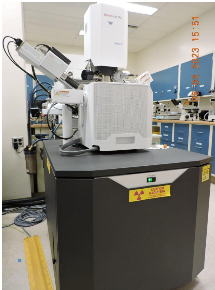
Figure 58. Environmental Scanning Electron Microscope Equipped with Several Detectors (ETD, CBS, ABS, GSED, LVD)
