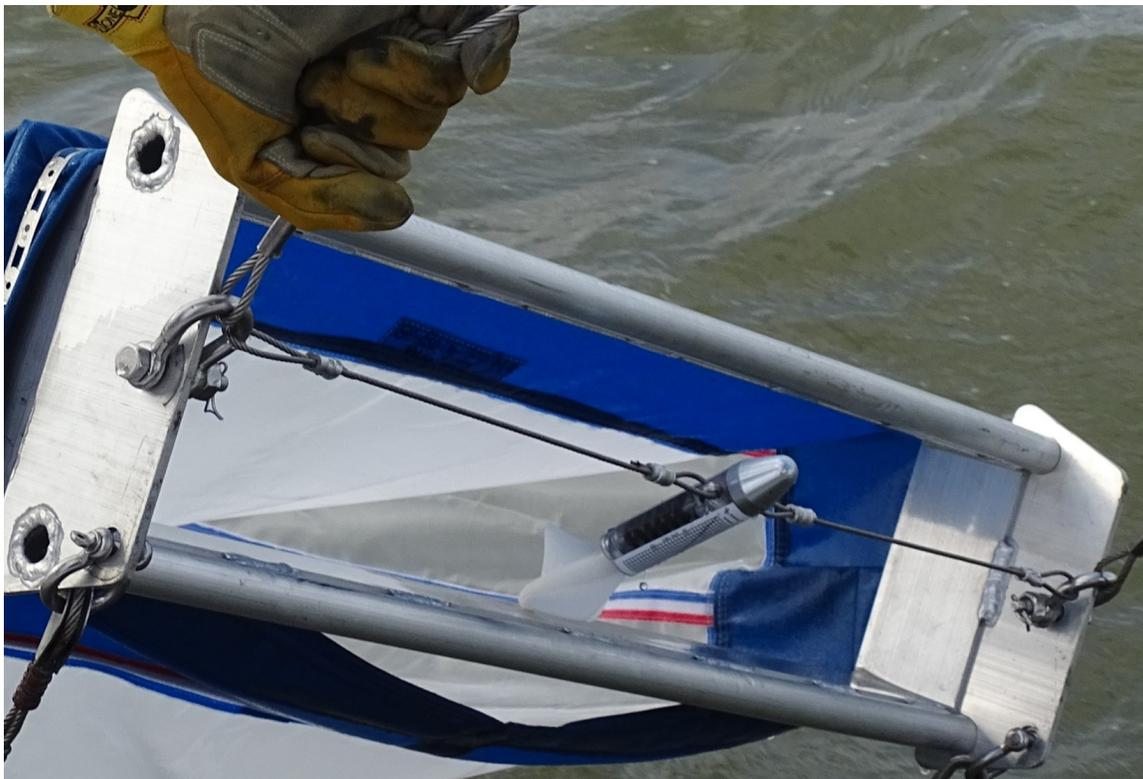
Figure 8. Flowmeter mounted in the net opening of the mid-depth net.
