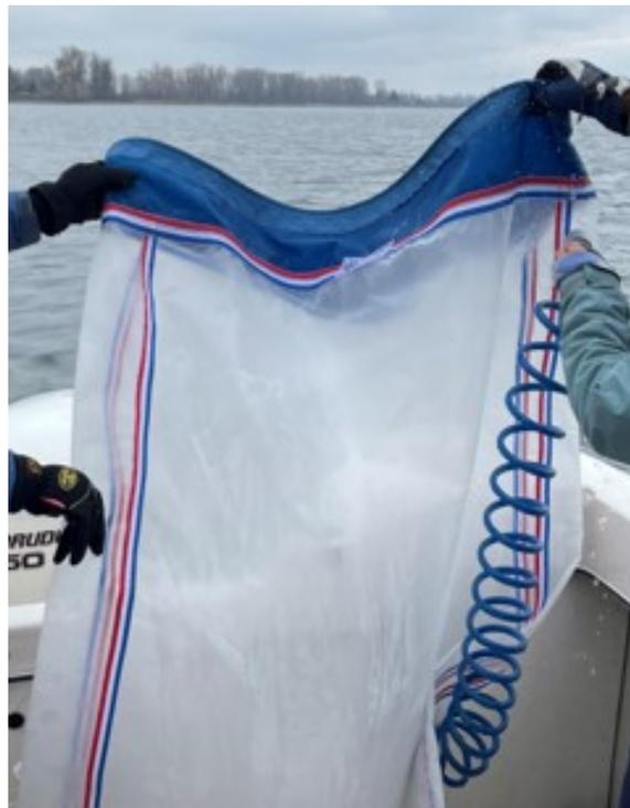
Figure 7. Rinsing the net with pumped river water.
