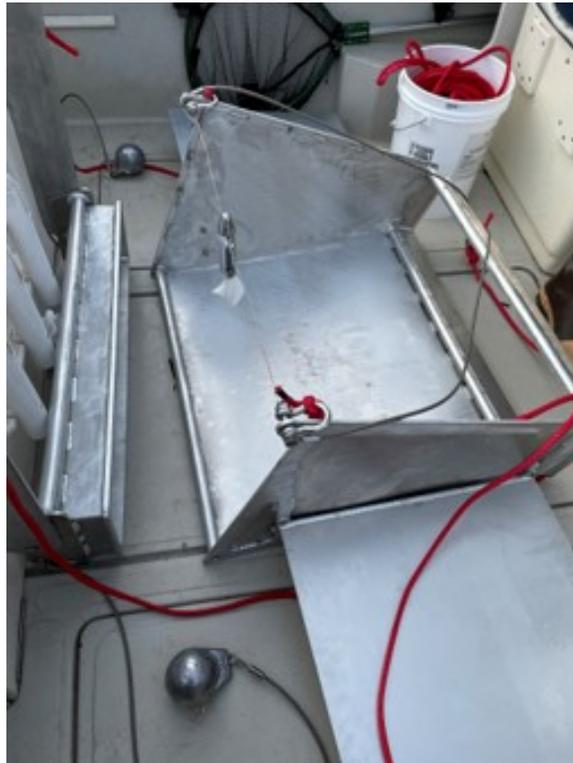
Figure 4. Net frames: mid-depth (left) and surface (right).
