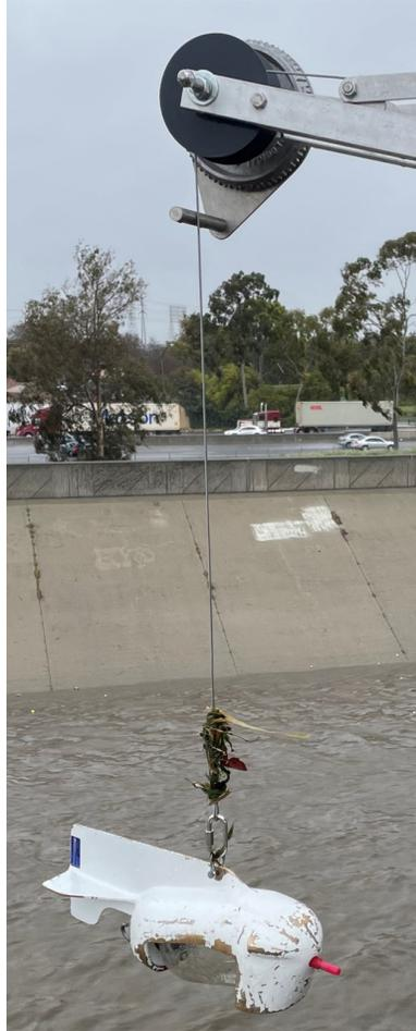
Figure 10. Whole water sampler used in the Los Angeles River.
