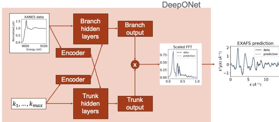
Figure 1: Diagram of the DeepONet
