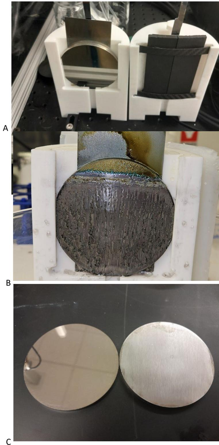
**Figure 7.** A) The demonstration piece and counter electrode. B) The plated workpiece prior to cleaning in ethanol and sonication. C) The original finish (left) and a coating of 35 μm of titanium (right).
