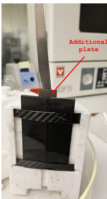
**Figure 5.** Auxiliary electrode part of the cell equipped with additional metal contact sheet.
