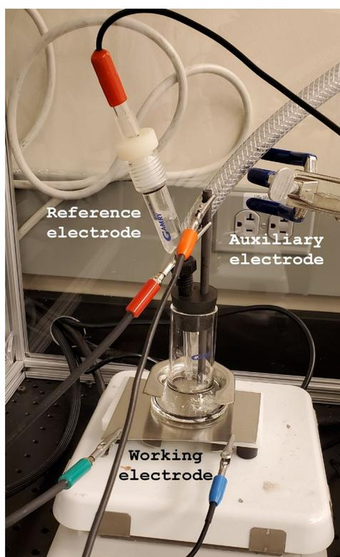
**Figure 2.** Fully assembled paint test cell.
