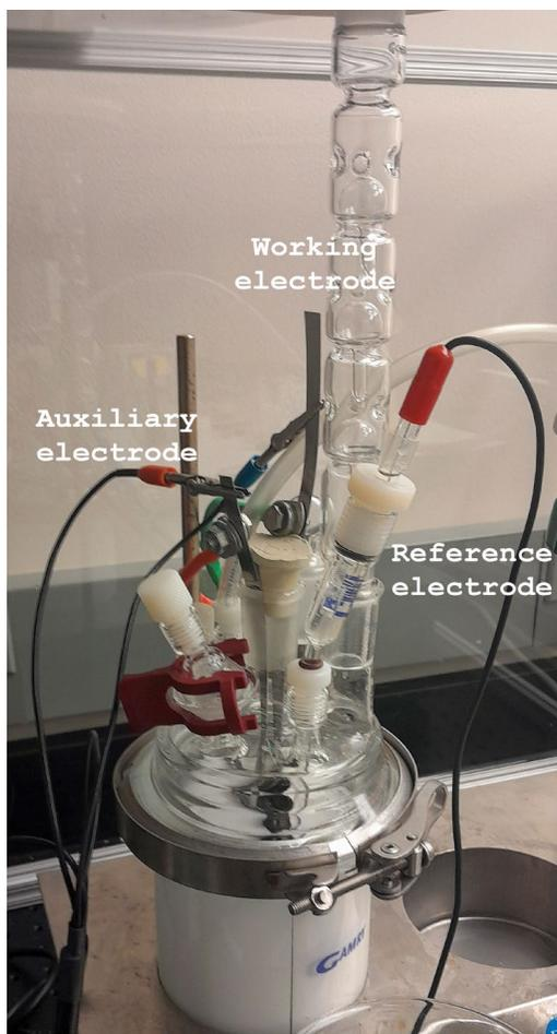
**Figure 4.** Fully assembled corrosion cell, equipped with condenser and Argon inlet (line in the back).
