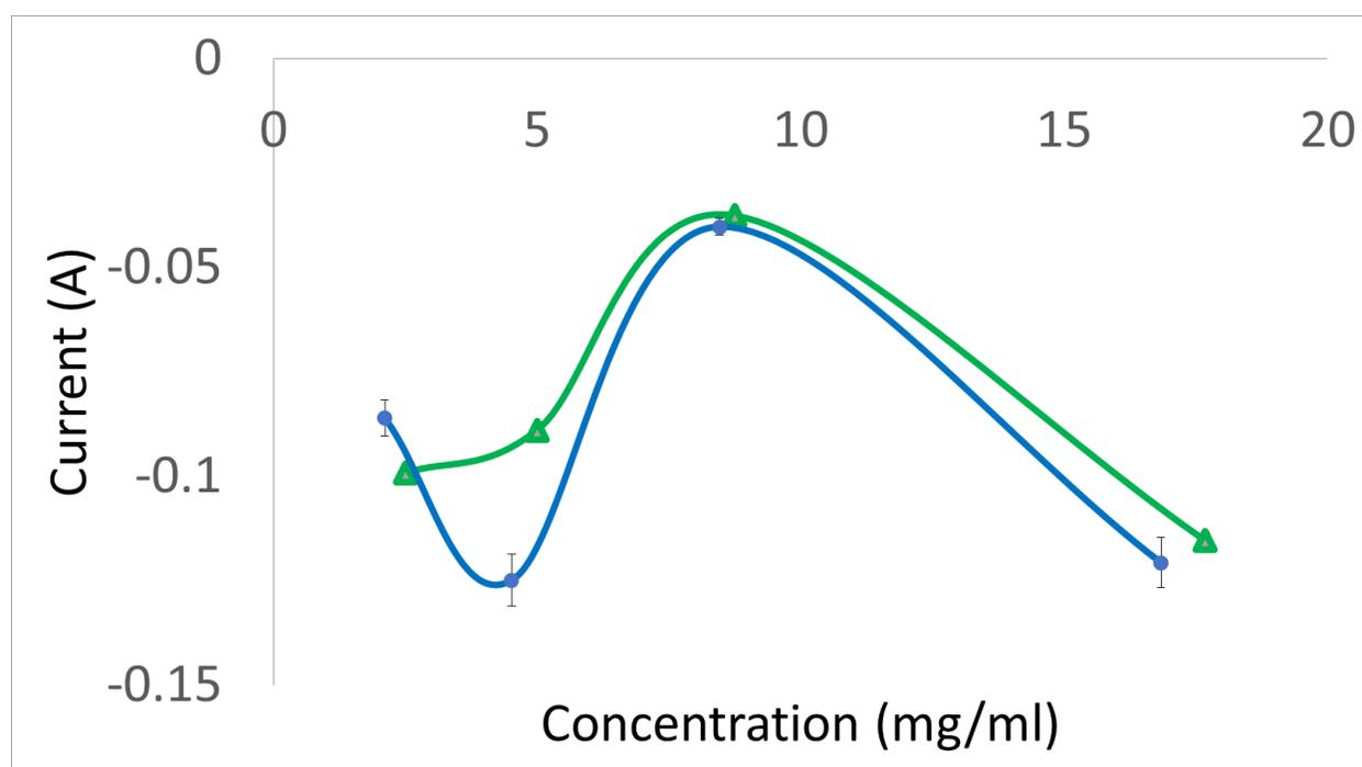
**Figure 1.** The behavior of  $\text{TiF}_4$  (green) compared to  $\text{TiF}_3$  (blue). The plating speed is largely the same between the two, though  $\text{TiF}_3$  is slightly faster at lower concentrations.
