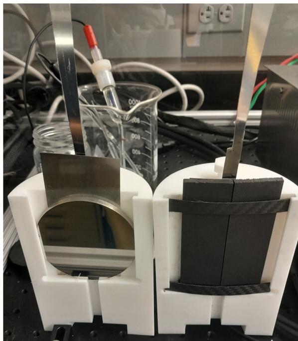
**Figure 3.** The two halves of the custom PTFE insert for the corrosion cell. The workpiece is on the left and the electrode is on the right.
