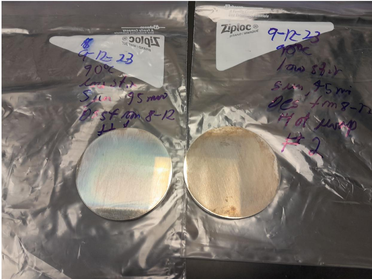
**Figure 6.** A demonstration piece plated at 40 °C showing 5  $\mu\text{m}$  thick titanium with oxide inclusions (left) and a hot-swapped piece plated at 60 °C showing 5  $\mu\text{m}$  of titanium metal (right).
