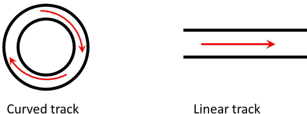
Figure 1. Schematic diagram of the curved and linear tracks. The arrows indicate the direction of ion motion inside the device.
