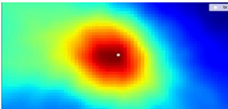
Figure 1. TDOA heatmap. The white dot represents the true transmitter location.
