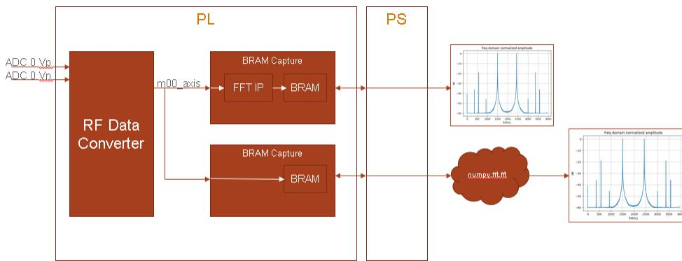
Figure 13. RFSoC test setup.
