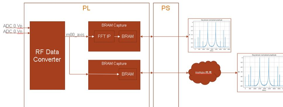
Figure 13. RFSoc test setup.
