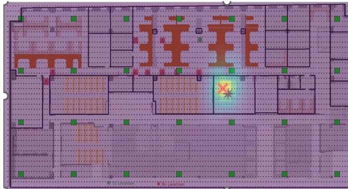
Figure 3. RSSI gaussian joint estimation heatmap.
