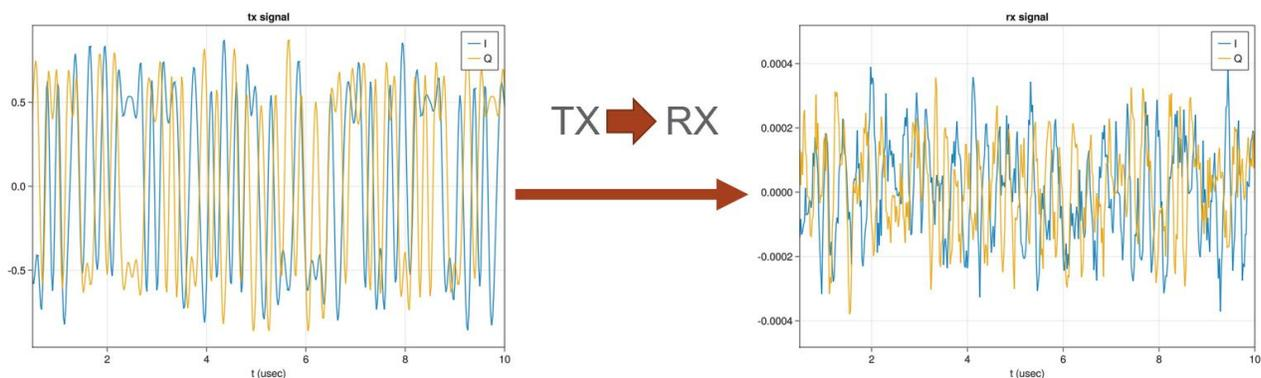
Figure 5. Transforming a transmit signal using the complex impulse response.
