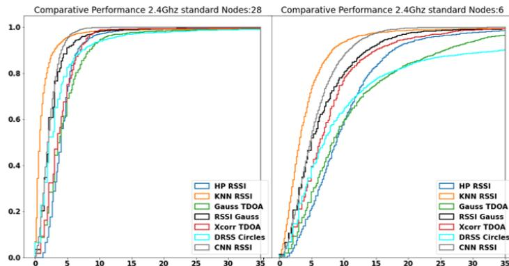
Figure 9. Cumulative error curve for each of the evaluated algorithms.
