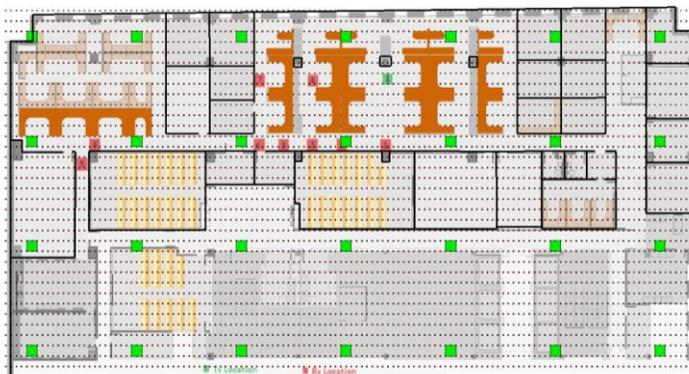
Figure 7. Simulation Test Bed, Green: RX, Red: TX
