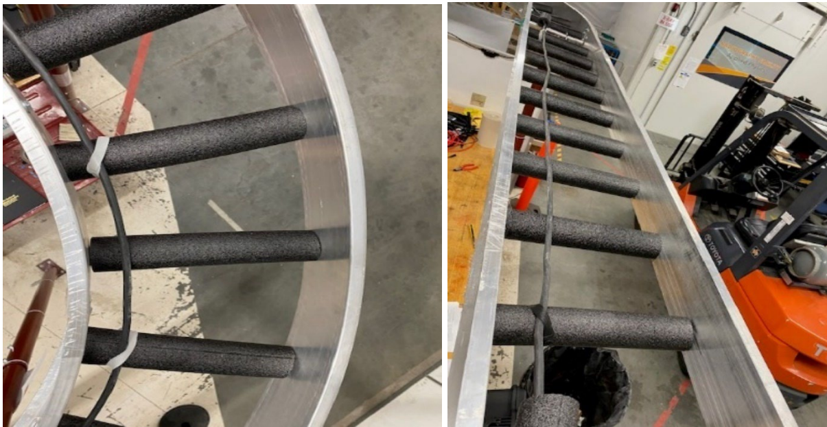
Figure 12. Unshielded cable resting on foam and separated from steel cable tray.
