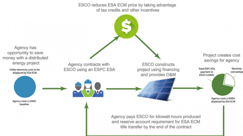
Figure 4. ESPC ESA financing system diagram with solar photovoltaic example (DOE - FEMP n.d.)
