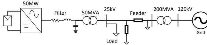
Figure 1: Tested system with 1-cluster of PV model.
