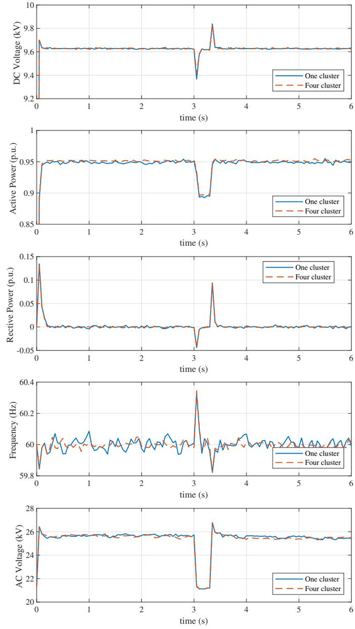
Figure 4: Simulation results under fault condition.
