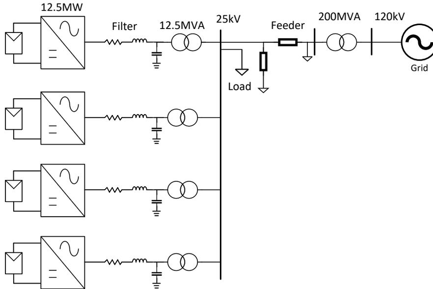
Figure 2: Tested system with 4-cluster of PV model.
