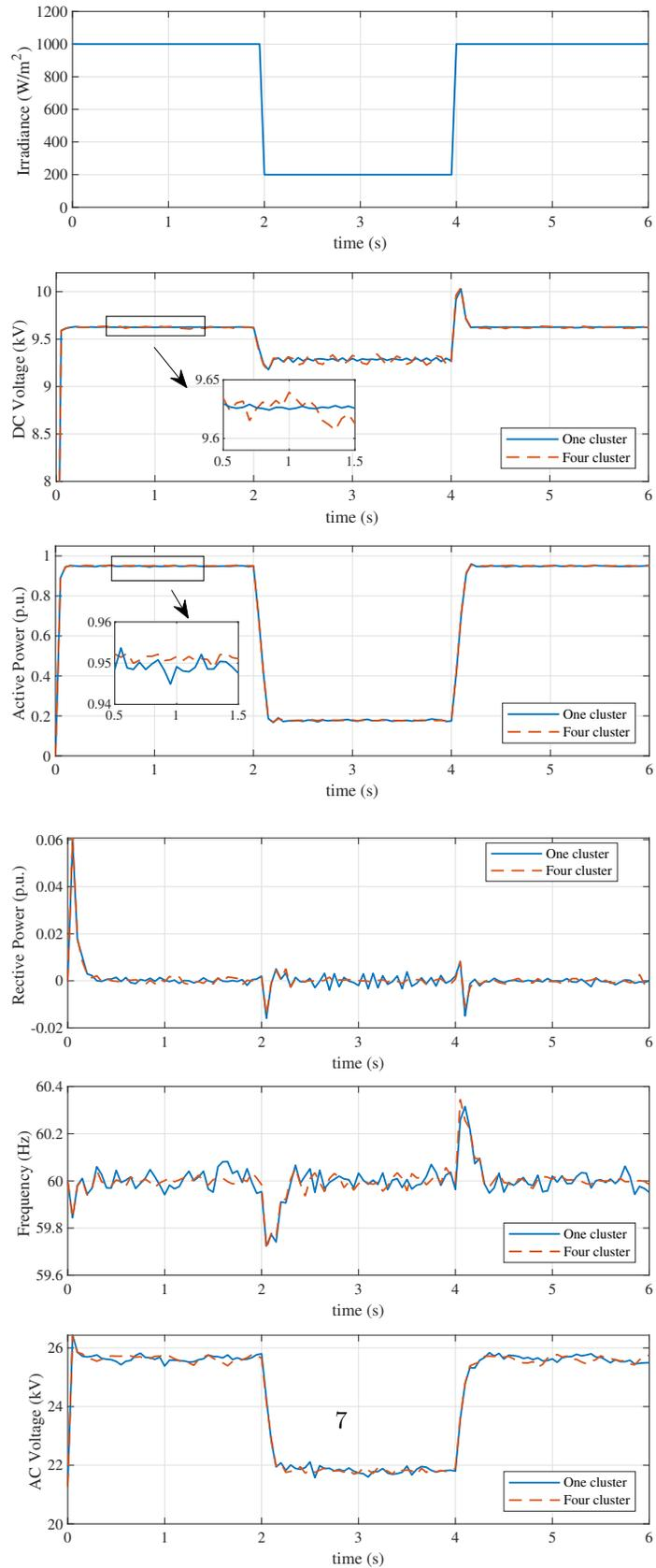
Figure 3: Simulation results under normal operation.
