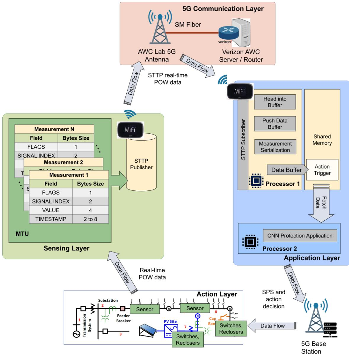
Figure 12 Diagram of 5G-enabled CNN-based learning protection scheme.
