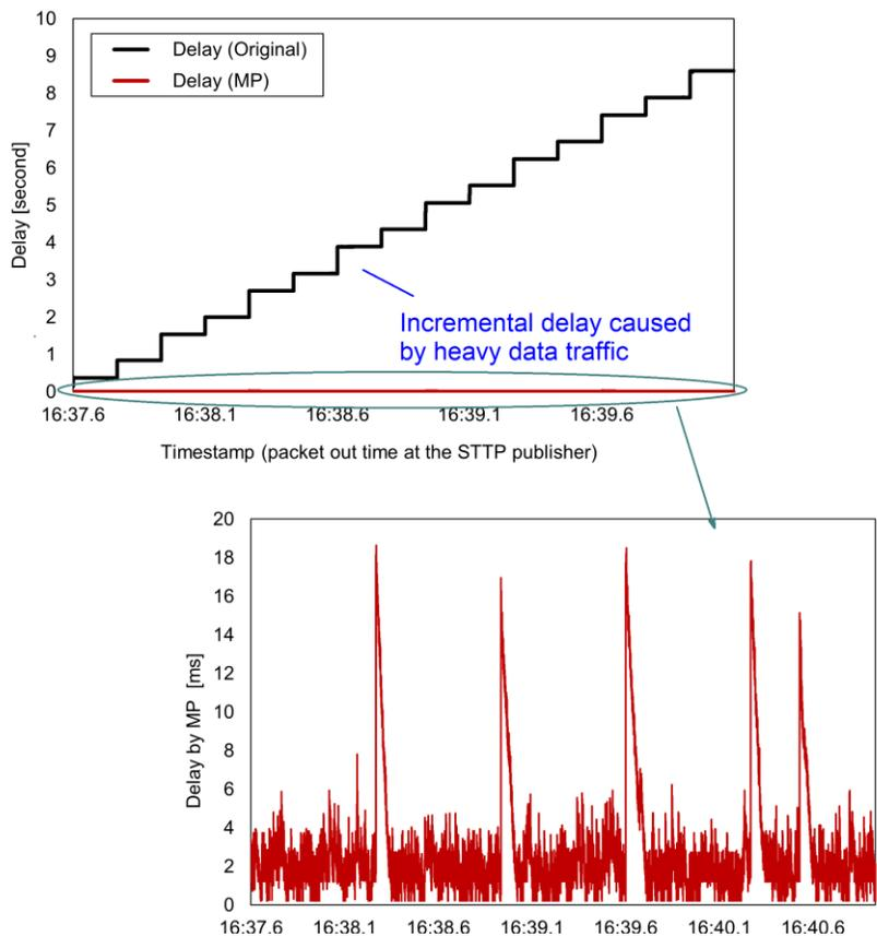
Figure 13 STTP data transmission delay was significantly reduced by mitigative serializing and multi-processing (MP) implementation.
