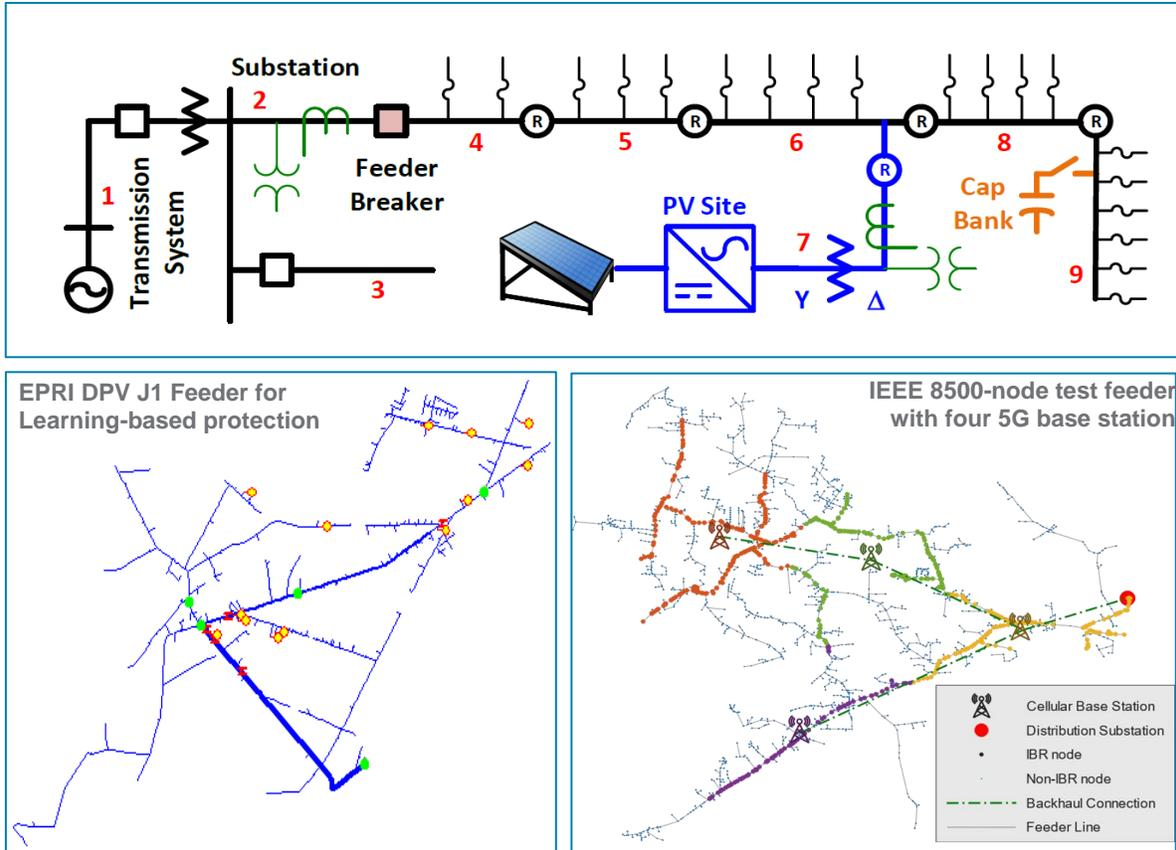
Figure 11 The learning-based protection for PV and two applicable test systems.
