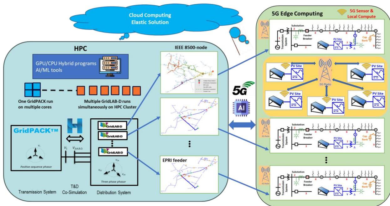
Figure 14 A detailed 5G-enabled power grid transmission, distribution, and communication co-simulation use case.
