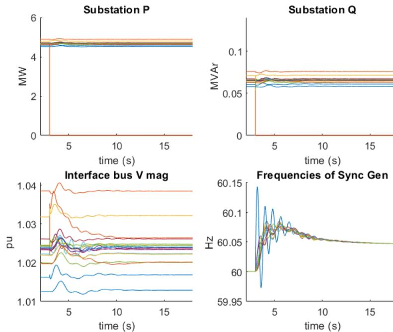
Figure 16 T&D co-simulation results: P, Q outputs at substation sides, voltage magnitude at the interface buses, as well as frequencies of synchronous generators at the transmission side.
