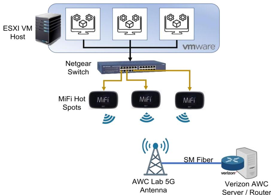
Figure 9 5G network configuration and VM settings for PMU, PDC, and PMU-based application.
