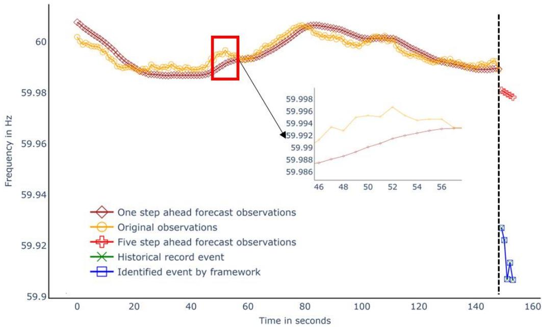
Figure 10 Detection of anomalous event at edge device using the PMU data stream via 5G network testbed.
