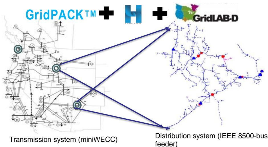
Figure 15 An Example of T&D co-simulation (the miniWECC transmission & nineteen IEEE 8500-node feeders)
