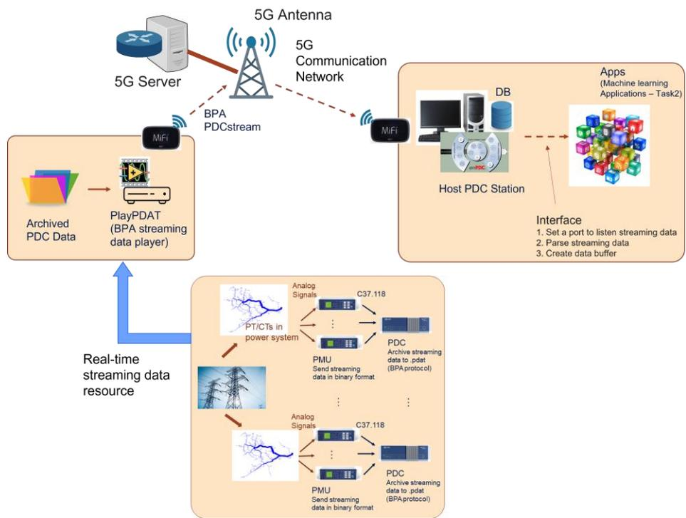
Figure 8 The simulation configuration for AI/ML example 1.
