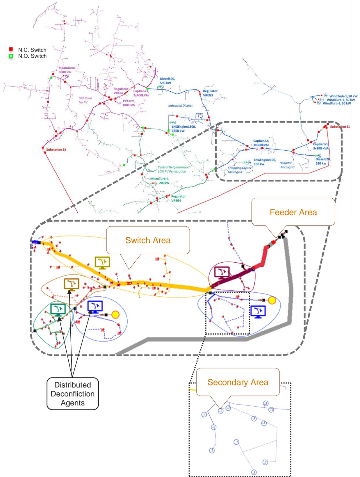
Figure 11: Decomposition of the 9500 Node Test System into individual switch areas and secondary areas
