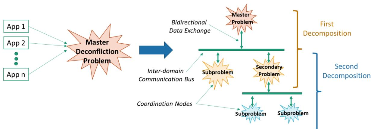
Figure 5: Decomposition of the application deconfliction problem using the Laminar Coordination Framework into subproblems handled by layered coordination nodes.
