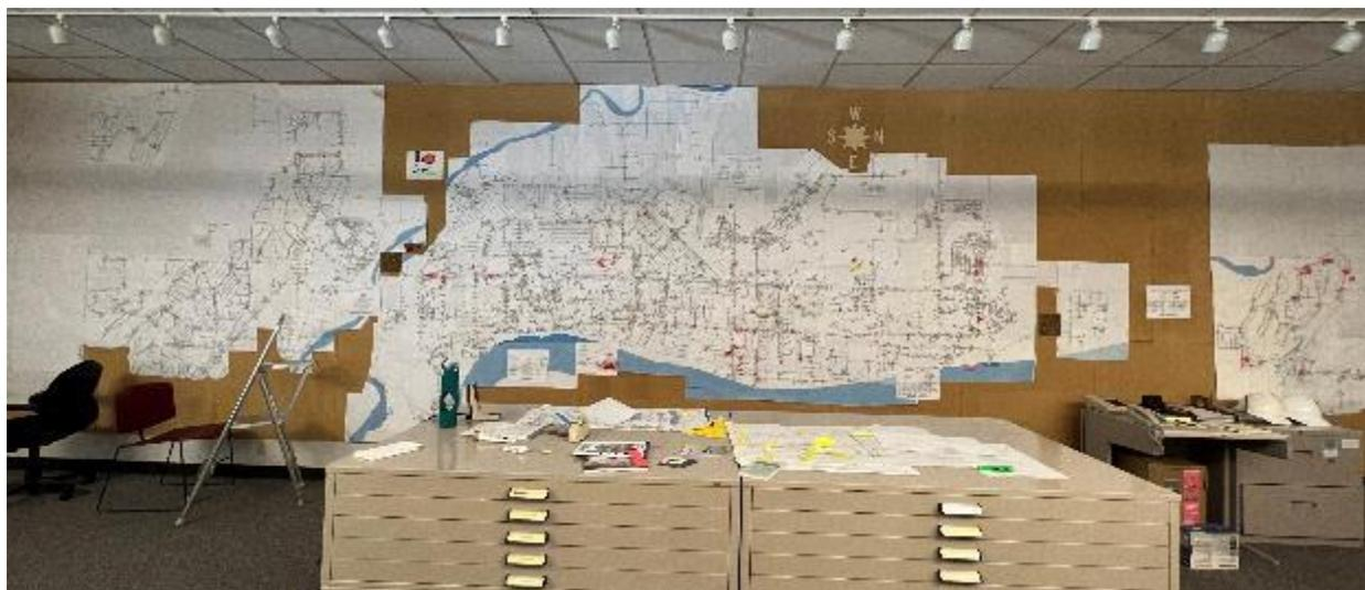
Figure 1: Operations wallboard of a municipal distribution utility with equipment positions and outages marked by colored flags on a geospatial map (courtesy Alka Singh & Rhonda Schennum)
