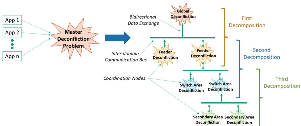
Figure 12: Decomposition iterations of the master deconfliction problem into individual subproblems limited to the controllable devices within each feeder, switch area, and secondary area.
