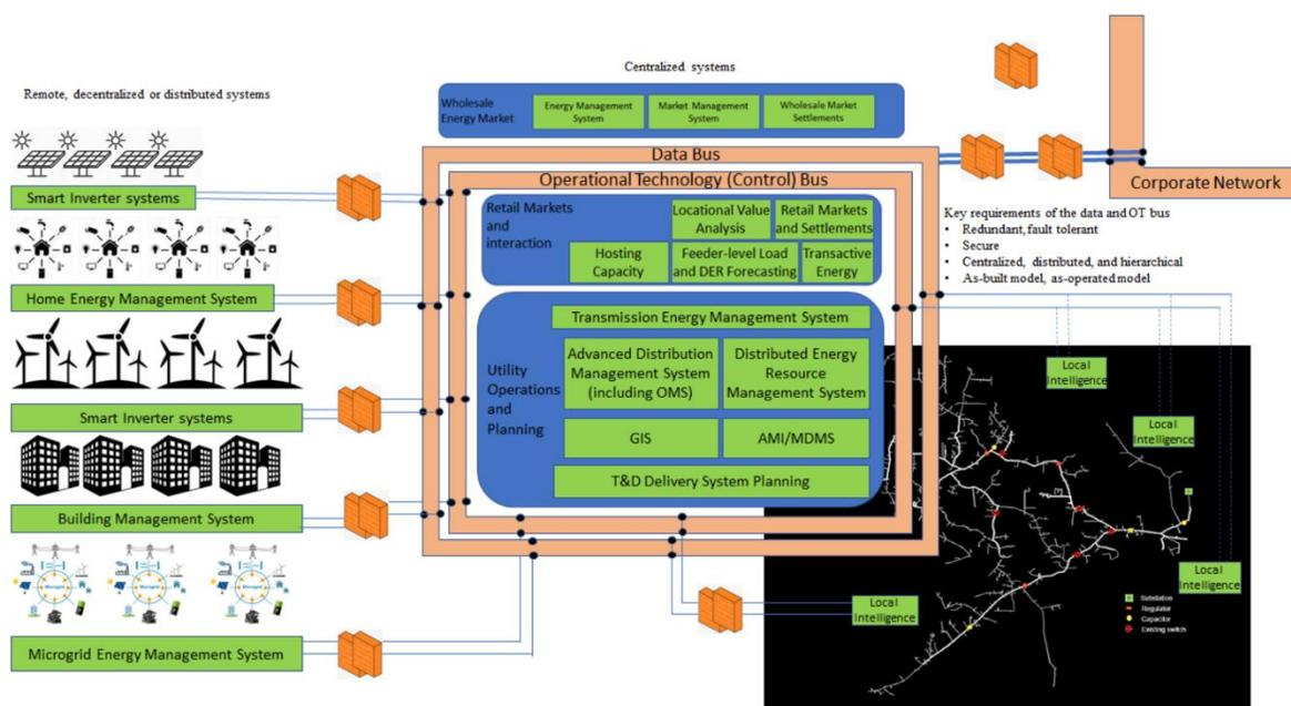
Figure 3: Conceptual separation of data flows onto an IT Data Bus and OT Control Bus, taken from [11]
