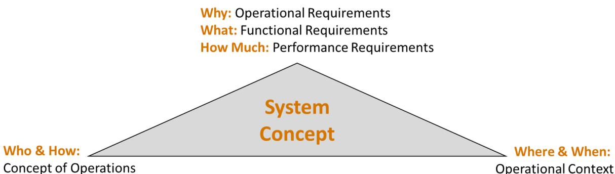
Figure 6: Triumvirate of Conceptual Design [14], which formulates seven interrogatives that form the basis of the requirements, operational context, and concept of operations.
