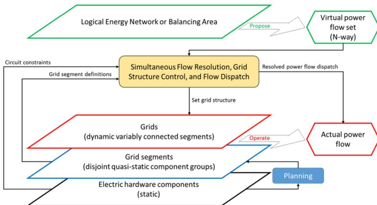
Figure 10: Decomposition of the distribution network into layers of a variable structure grid, taken from [8]
