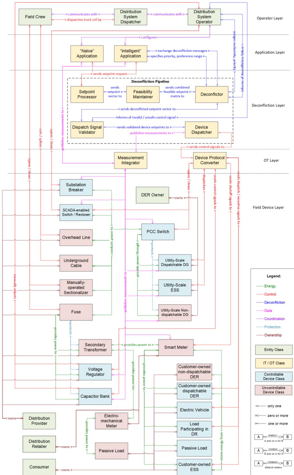
Figure 7: Entity structure diagram illustrating relationships between key stakeholders, IT / OT processes, and field devices
