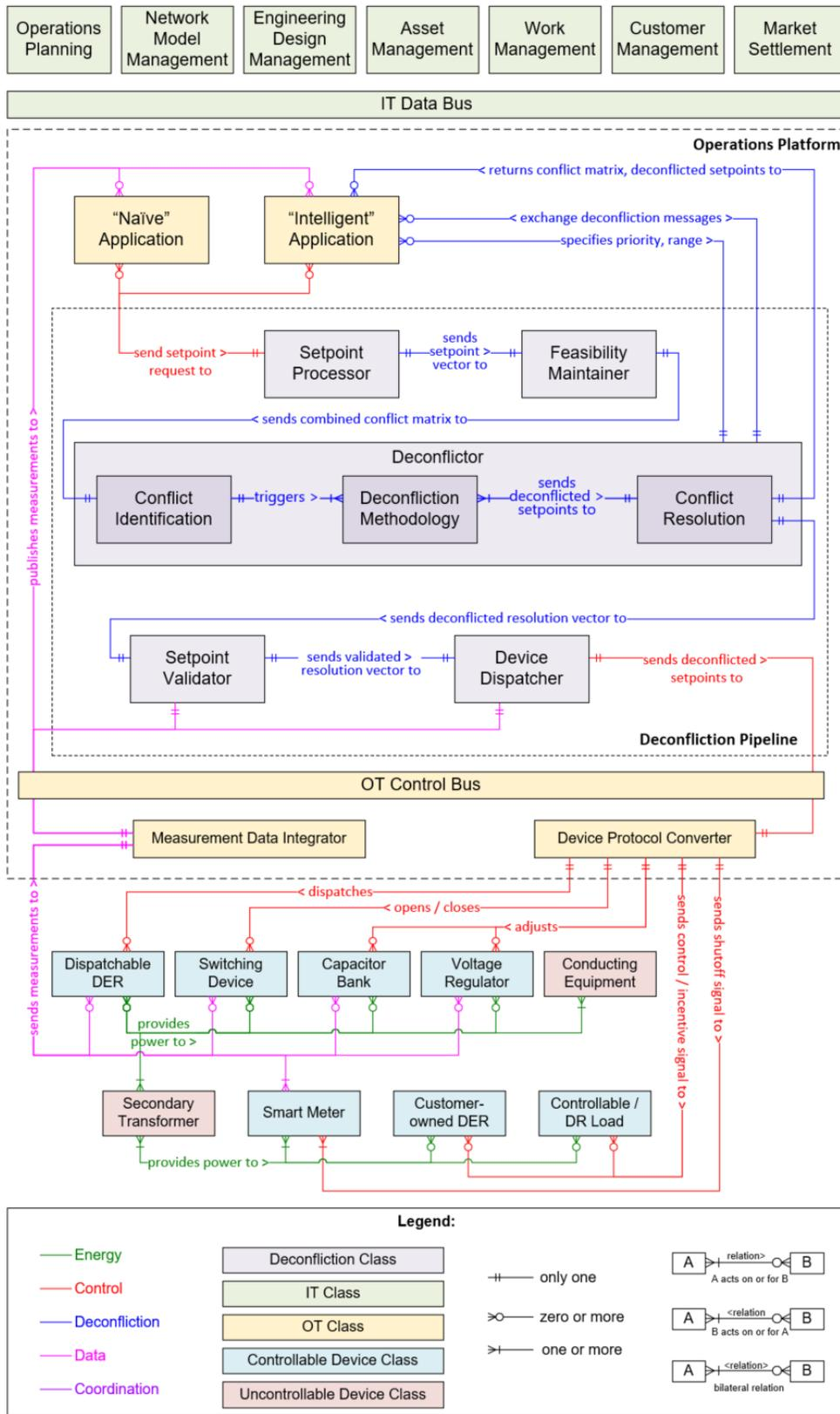
Figure 4: Deconfliction Pipeline for identifying and resolving conflicting setpoints issued by advanced power applications
