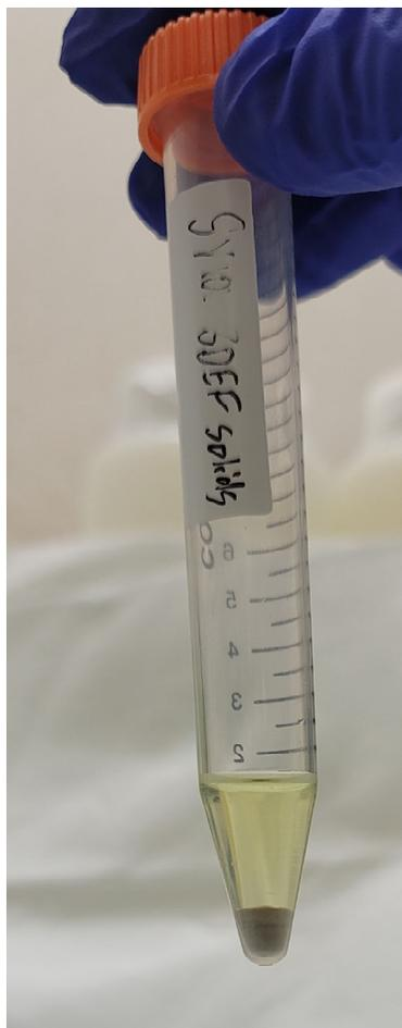
Figure 3.6. Concentrated solids in fumehood after centrifuging.
