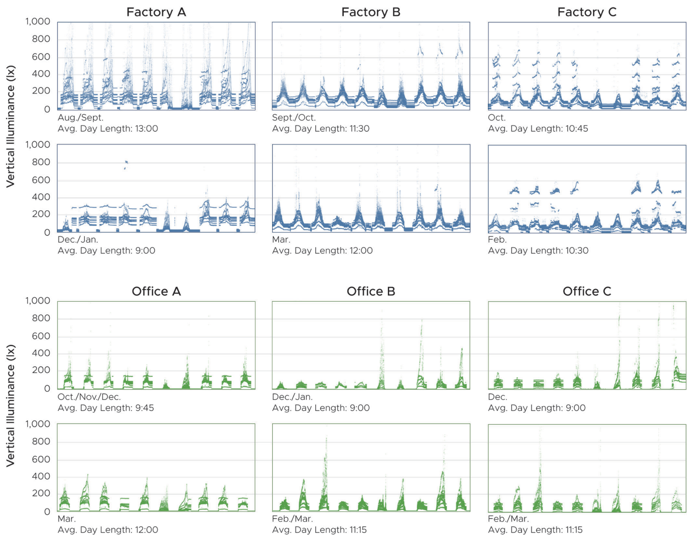
Figure 4: Sample of time-series data for all vertical measurement locations. All time-series plots begin on a Monday; the plots include weekends to show the difference between workdays and weekends.
