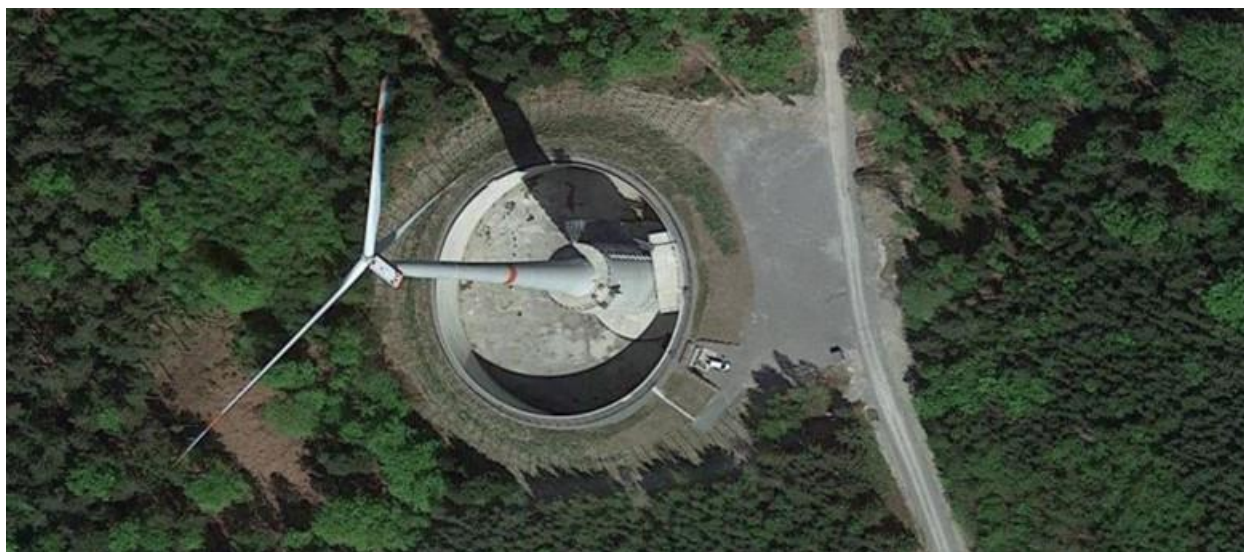
Figure 20. Satellite image of combined wind turbine foundation and PSH upper reservoir at the Gaildorf pilot hybrid PSH-wind facility in Germany (Image: Google Maps).
