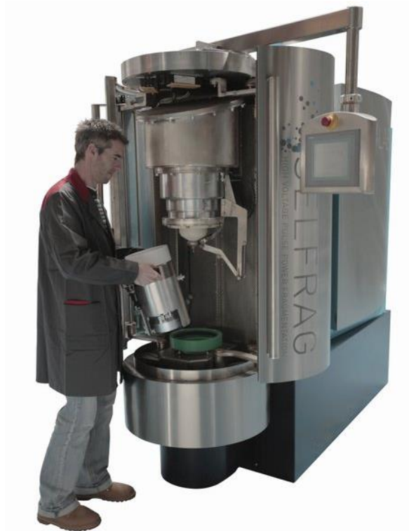
Figure 6-1. SELFRAG Laboratory Fragmenter. The unit is entirely self-contained and operated by a remote touchscreen.
