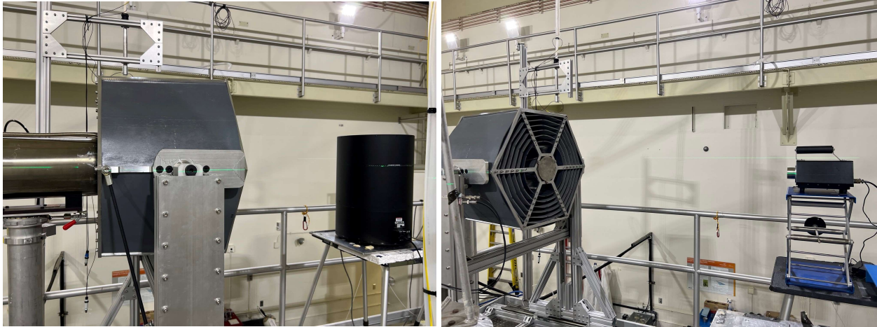
Figure 16. The SSA prototype field measured with ROSPEC (left) and SSS probe (right).
