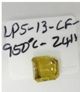
Figure G.15. Glass LP5-13 after CF Heat Treatment at 950 °C for 24 Hours
