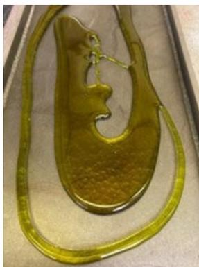
Figure D.37. Photo of Glass LAW-HPVR-12 Morphology after the Second Melt
