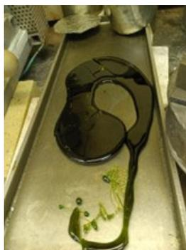
Figure D.1. Glass LP5-01 Morphology after the Second Melt
