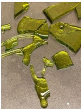
Figure D.44. Photo of Glass LAW-HPVR-19 Morphology after the Second Melt
