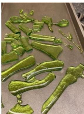
Figure D.36. Photo of Glass LAW-HPVR-11 Morphology after the Second Melt
