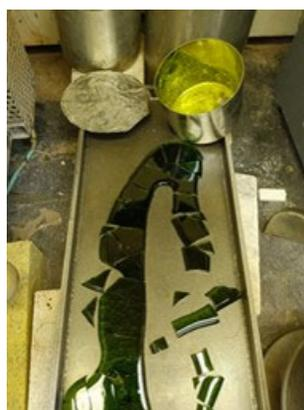
Figure D.2. Glass LP5-02 Morphology after the Second Melt
