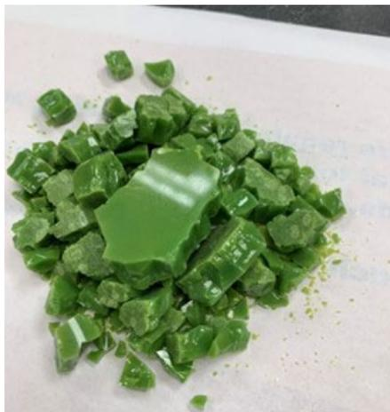
Figure F.8. Glass LP5-06-MOD1 Morphology after CCC. The quantity of the crystals was too low to be identified by XRD.
