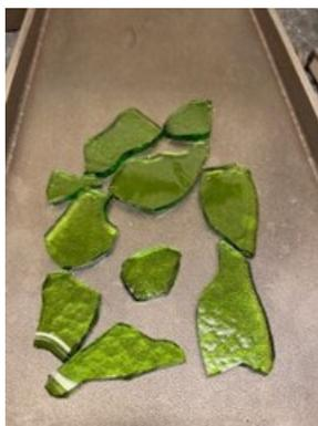
Figure D.32. Photo of Glass LAW-HPVR-07 Morphology after the Third Melt
