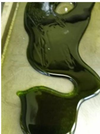
Figure D.13. Photo of Glass LP5-13 Morphology after the Second Melt
