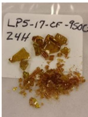
Figure G.20. Glass LP5-17 after CF Heat Treatment at 950 °C for 24 Hours
