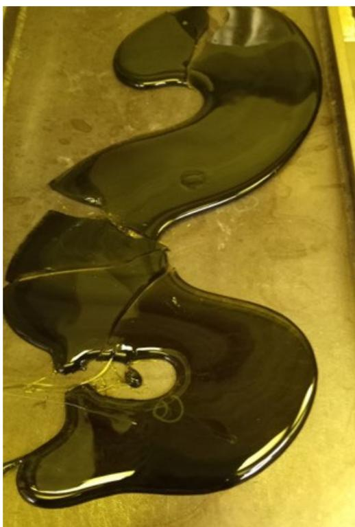
Figure 2.2. LP5-16 Glass Fifth Melt at 1350 °C
