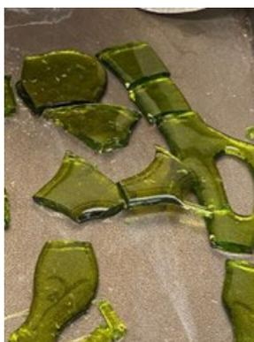
Figure D.45. Photo of Glass LAW-HPVR-20 Morphology after the Second Melt
