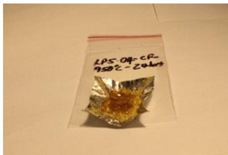
Figure G.4. Glass LP5-04 after CF Heat Treatment at 950 °C for 24 Hours
