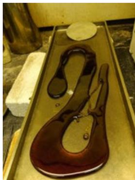
Figure D.3. Glass LP5-03 Morphology after the Second Melt
