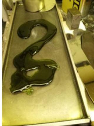
Figure D.22. Photo of Glass LP5-22 Morphology after the Second Melt
