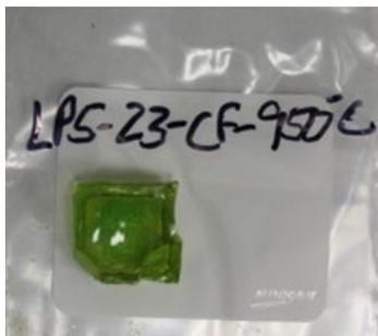
Figure G.26. Glass LP5-23 after CF Heat Treatment at 950 °C for 24 Hours
