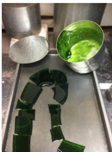
Figure D.6. Glass LP5-06-mod1 Morphology after the Third Melt
