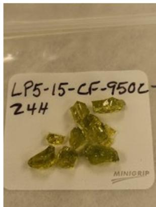
Figure G.17. Glass LP5-15 after CF Heat Treatment at 950 °C for 24 Hours
