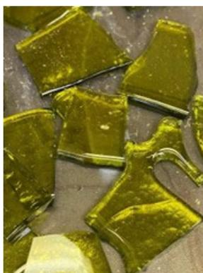
Figure D.33. Photo of Glass LAW-HPVR-08 Morphology after the Second Melt
