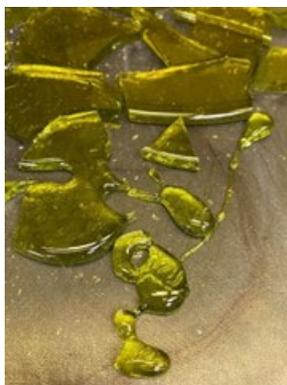
Figure D.28. Photo of Glass LAW-HPVR-03-1 Morphology after the Third Melt
