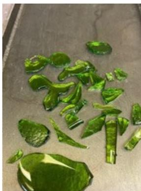
Figure D.50. Photo of Glass LAW-HPVR-25 Morphology after the Third Melt
