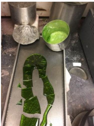
Figure D.7. Photo of Glass LP5-07 Morphology of the Third Melt
