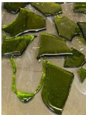
Figure D.47. Photo of Glass LAW-HPVR-22 Morphology after the Third Melt
