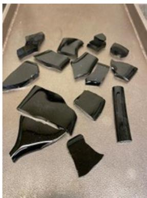
Figure D.43. Photo of Glass LAW-HPVR-18 Morphology after the Second Melt
