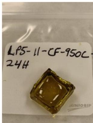
Figure G.12. Glass LP5-11 after CF Heat Treatment at 950 °C for 24 Hours
