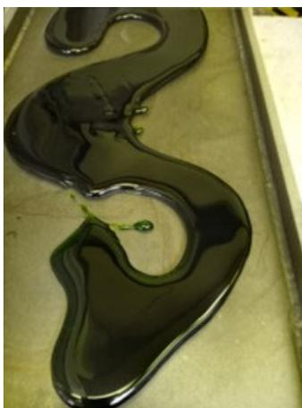
Figure D.21. Photo of Glass LP5-21 Morphology after the Second Melt
