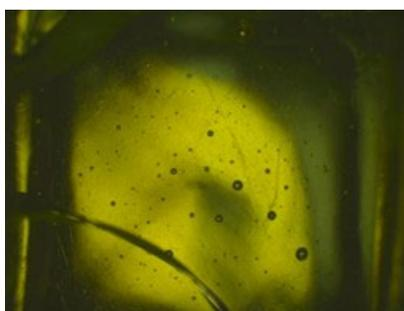
Figure G.7. Glass LP5-07 after CF Heat Treatment at 950 °C for 24 Hours
