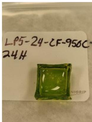
Figure G.27. Glass LP5-24 after CF Heat Treatment at 950 °C for 24 Hours
