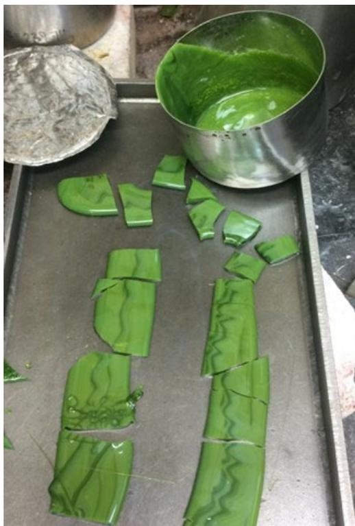
Figure 2.1. LP5-06 Glass Fourth Melt at 1350 °C
