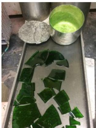
Figure D.4. Glass LP5-04 Morphology after the Second Melt
