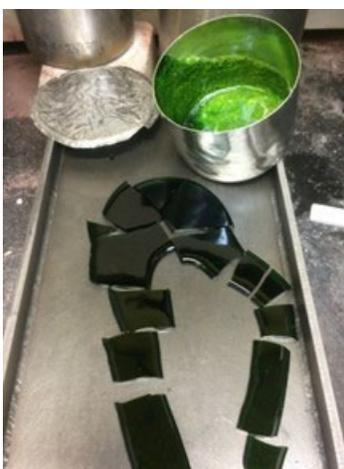
Figure D.20. Photo of Glass LP5-20 Morphology after the Second Melt
