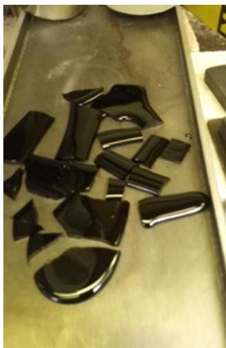
Figure D.25. Photo of Glass LP5-25 Morphology after the Third Melt
