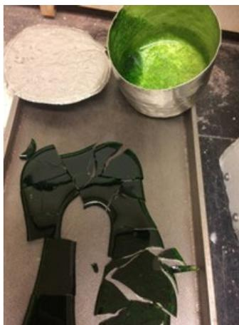
Figure D.18. Photo of Glass LP5-18 Morphology after the Third Melt
