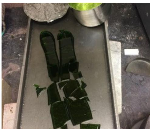
Figure D.5. Glass LP5-05 Morphology after the Second Melt
