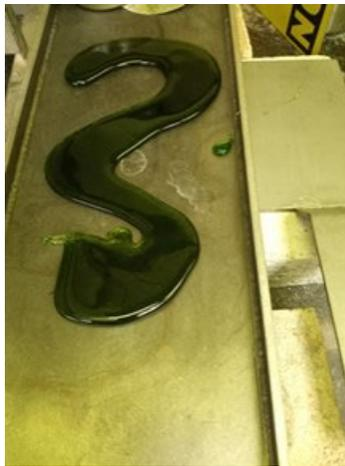
Figure D.23. Photo of Glass LP5-23 Morphology after the Second Melt
