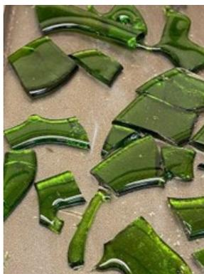
Figure D.49. Photo of Glass LAW-HPVR-24 Morphology after the Second Melt
