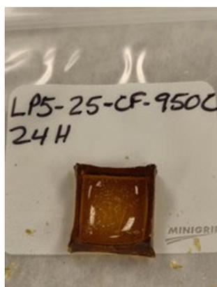
Figure G.28. Glass LP5-25 after CF Heat Treatment at 950 °C for 24 Hours
