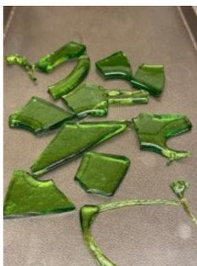
Figure D.48. Photo of Glass LAW-HPVR-23 Morphology after the Second Melt
