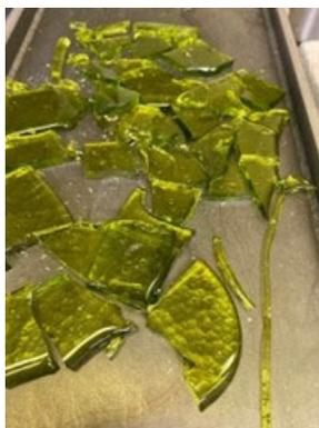
Figure D.31. Photo of Glass LAW-HPVR-06 Morphology after the Second Melt
