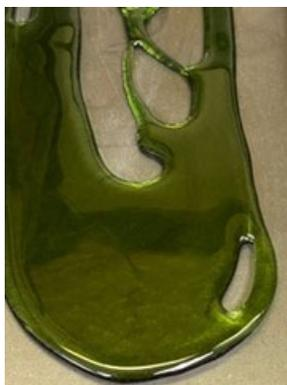
Figure D.40. Photo of Glass LAW-HPVR-15 Morphology after the Second Melt
