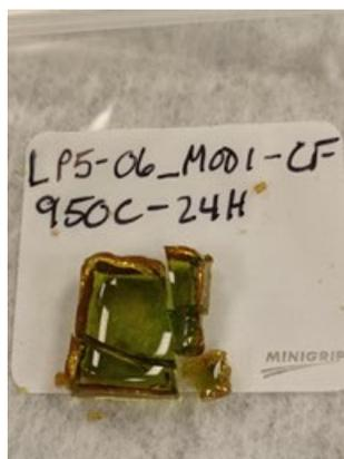
Figure G.6. Glass LP5-06-MOD1 after CF Heat Treatment at 950 °C for 24 Hours
