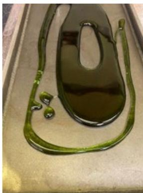
Figure D.35. Photo of Glass LAW-HPVR-10 Morphology after the Second Melt
