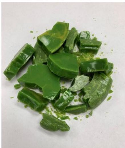
Figure F.15. Glass LP5-11 Morphology after CCC. The quantity of the crystals was too low to be identified by XRD.
