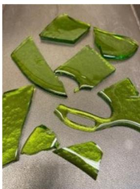
Figure D.42. Photo of Glass LAW-HPVR-17 Morphology after the Second Melt
