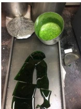
Figure D.8. Photo of Glass LP5-08 Morphology of the Second Melt
