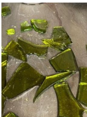
Figure D.39. Photo of Glass LAW-HPVR-14 Morphology after the Second Melt
