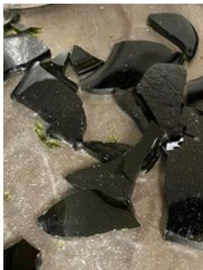
Figure D.27. Photo of Glass LAW-HPVR-02-1 Morphology after the Second Melt
