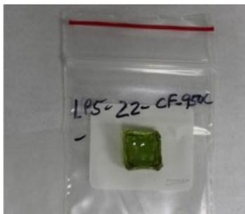
Figure G.25. Glass LP5-22 after CF Heat Treatment at 950 °C for 24 Hours
