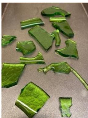
Figure D.51. Photo of Glass LAW-HPVR-26 Morphology after the Second Melt
