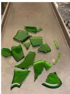
Figure D.30. Photo of Glass LAW-HPVR-05 Morphology after the Second Melt
