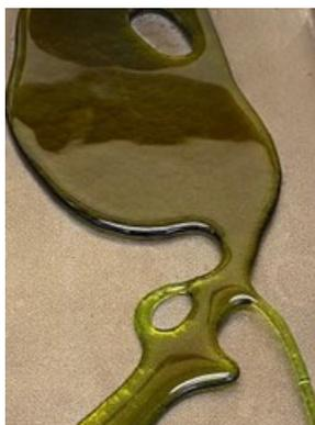
Figure D.41. Photo of Glass LAW-HPVR-16 Morphology after the Second Melt
