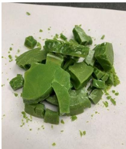
Figure F.19. Glass LP5-14 Morphology after CCC. The quantity of the crystals was too low to be identified by XRD.
