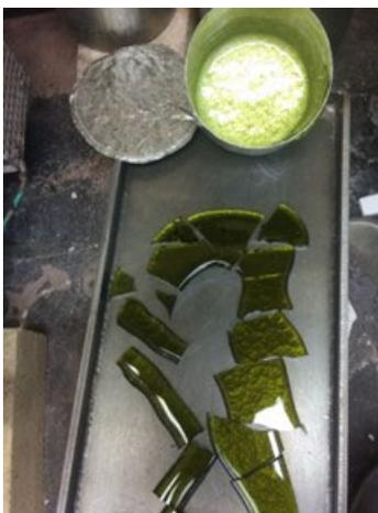
Figure D.15. Photo of Glass LP5-15 Morphology after the Forth Melt
