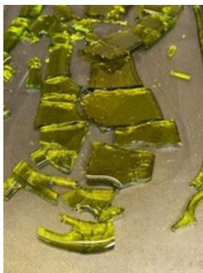
Figure D.46. Photo of Glass LAW-HPVR-21 Morphology after the Second Melt
