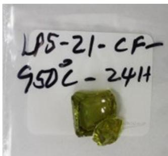
Figure G.24. Glass LP5-21 after CF Heat Treatment at 950 °C for 24 Hours
