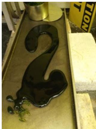
Figure D.14. Photo of Glass LP5-14 Morphology after the Third Melt
