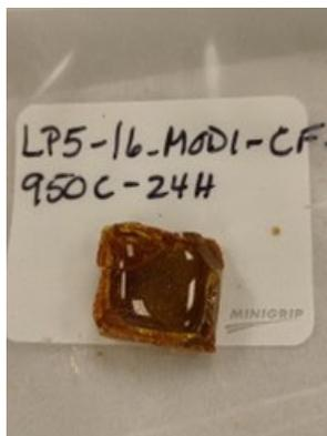
Figure G.18. Glass LP5-16-MOD1 after CF Heat Treatment at 950 °C for 24 Hours
