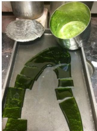
Figure D.17. Photo of Glass LP5-17 Morphology after the Forth Melt
