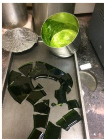
Figure D.11. Photo of Glass LP5-11 Morphology of the Third Melt
