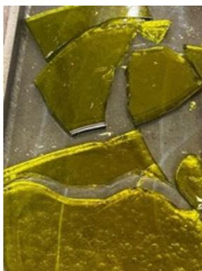
Figure D.26. Photo of Glass LAW-HPVR-01-1 Morphology after the Second Melt
