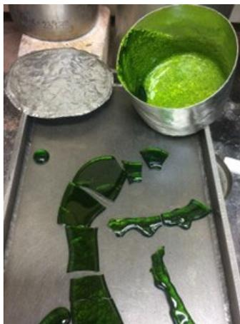
Figure D.24. Photo of Glass LP5-24 Morphology after the Third Melt
