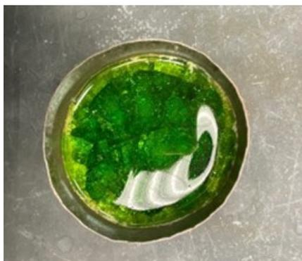
Figure F.45. Glass LAW-HPVR-14 Morphology after CCC. The quantity of the crystals was too low to be identified by XRD.
