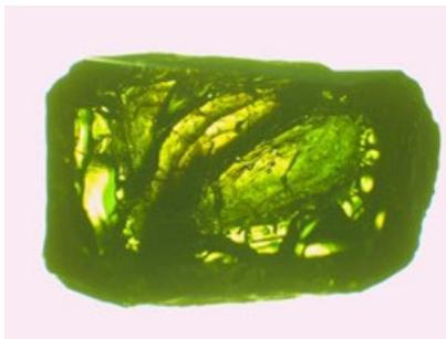
Figure G.8. Glass LP5-08 after CF Heat Treatment at 950 °C for 24 Hours
