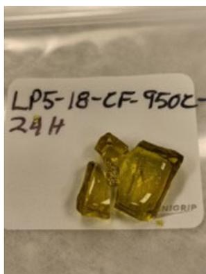
Figure G.21. Glass LP5-18 after CF Heat Treatment at 950 °C for 24 Hours
