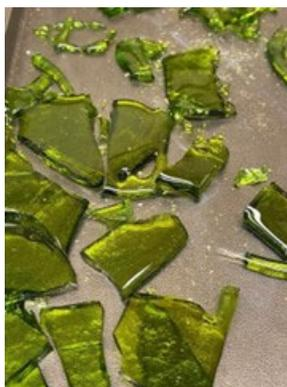
Figure D.38. Photo of Glass LAW-HPVR-13 Morphology after the Third Melt
