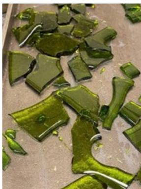
Figure D.29. Photo of Glass LAW-HPVR-04-1 Morphology after the Second Melt
