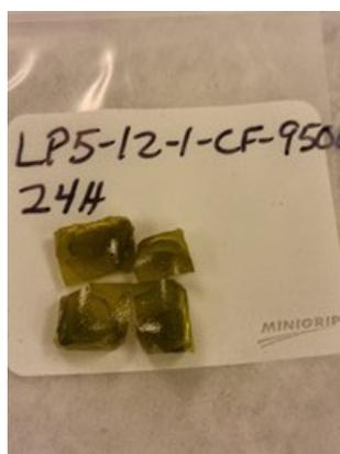
Figure G.13. Glass LP5-12-1 after CF Heat Treatment at 950 °C for 24 Hours
