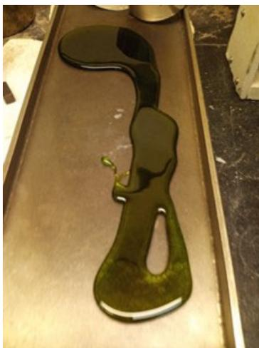
Figure D.10. Photo of Glass LP5-10 Morphology of the Second Melt
