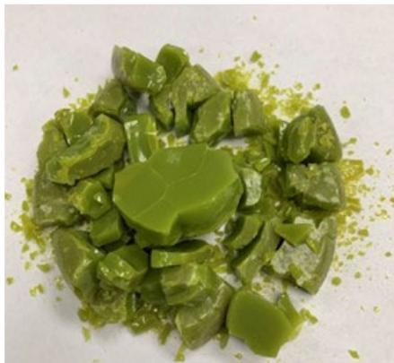
Figure F.4. Glass LP5-03 Morphology after CCC. The quantity of the crystals was too low to be identified by XRD.
