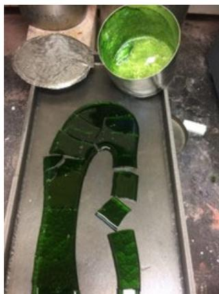
Figure D.19. Photo of Glass LP5-19 Morphology after the Second Melt
