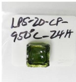
Figure G.23. Glass LP5-20 after CF Heat Treatment at 950 °C for 24 Hours
