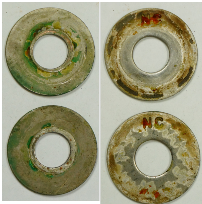
Figure 5.26. Exterior (left) and Interior (right) surface condition Monel alloy – Hybrid composite
