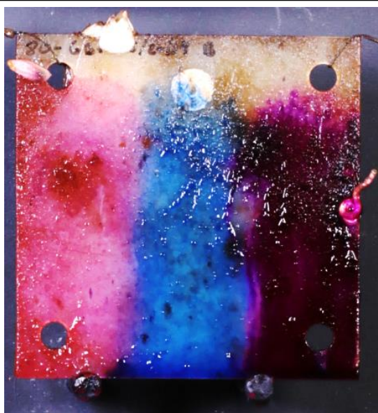
Figure 4.2. Image showing each of the stain components applied individually to strips of a fouled sample coupon. The three stains (From left to right, Erythrosin B [stains basic structures], Coomassie G-250 [stains proteins and amino acids] and Rhodamine WT [stains biofilm retained water]) each stain various different components of the biofilm, but can also each be used to determine a BGI value. The combination of the three allow greater sample surface variability (e.g., color variations) while maintaining quantifiability of the extent of fouling.
