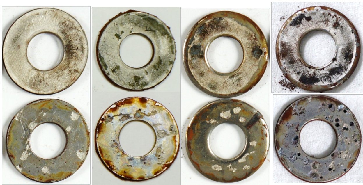
Figure 5.16. Exterior washer surface condition from specimens SS-CF immersed in ET tank
