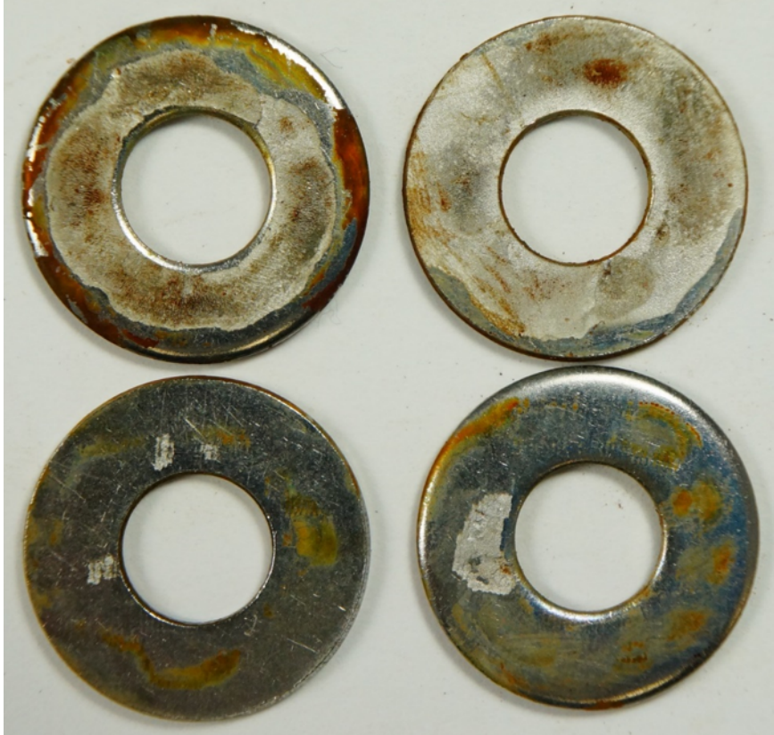
Figure 5.8 Washers SS-RT interior surface
