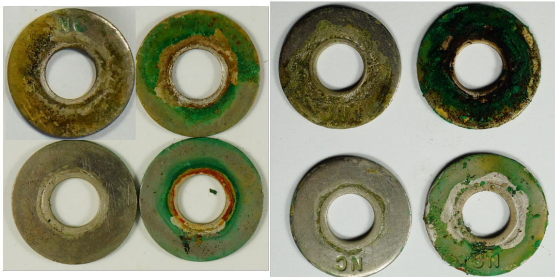
Figure 5.19. Exterior surface condition Monel-CF
