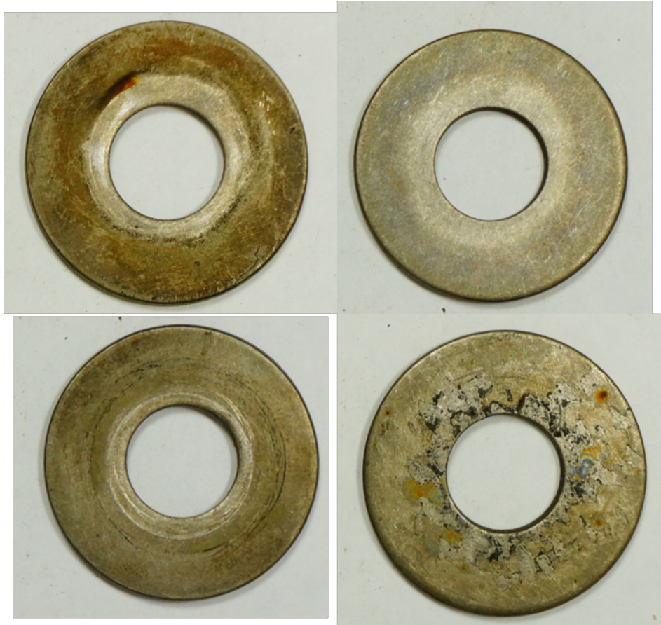
Figure 5.27. Exterior (left) and Interior (right) surface condition Ti – Hybrid composite SEM
