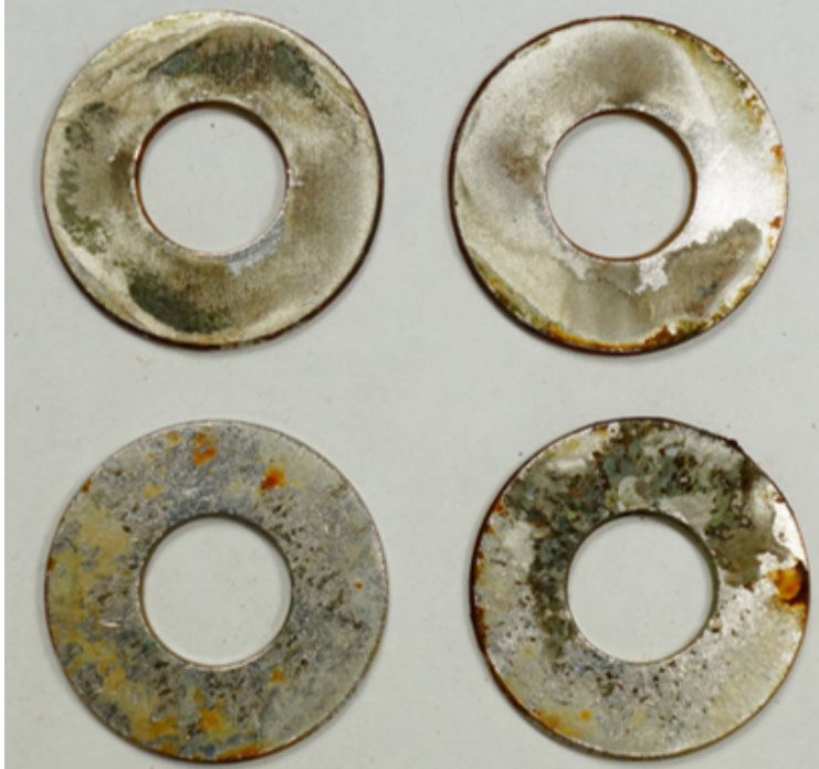
Figure 5.25. Interior surface condition SS – Hybrid composite (immersed in seawater ET)
