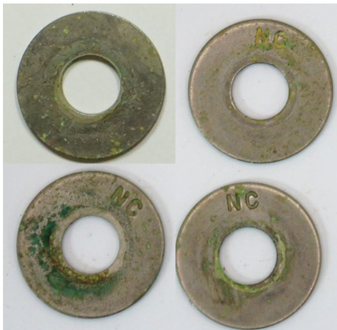
Figure 5.10. Washer Monel/CF RT exterior surface
