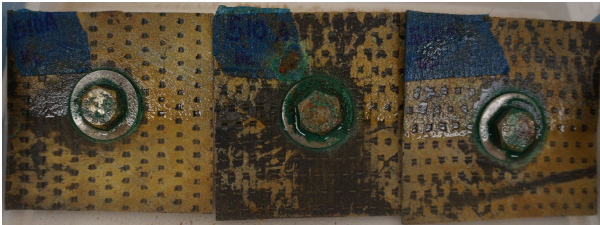
Figure 5.6 Elevated temperature exposed Monel/CF specimens after 273 days of immersion
