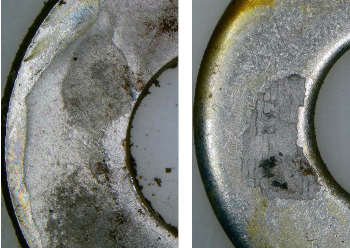
Figure 5.9. RT-SS Washer surface in contact with composite: left smooth side and right rougher side.
