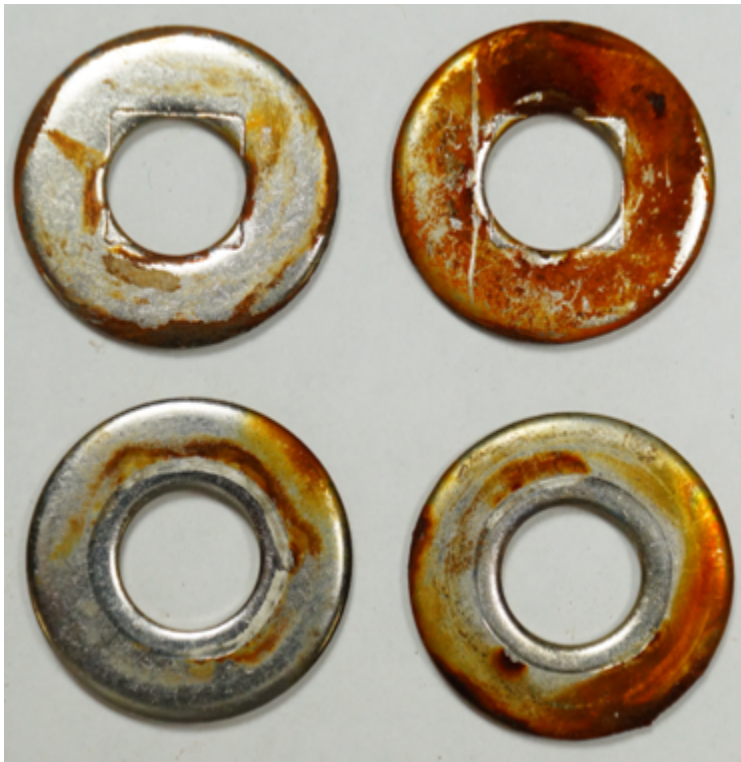
Figure 5.24. Exterior surface condition SS – Hybrid composite (immerse in seawater ET)
