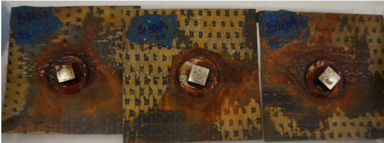
Figure 5.5 Elevated temperature exposed SS/CF specimens after 273 days of immersion
