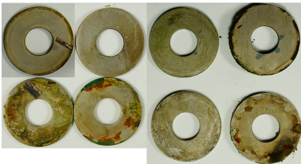
Figure 5.20. Interior surface condition Monel-CF
