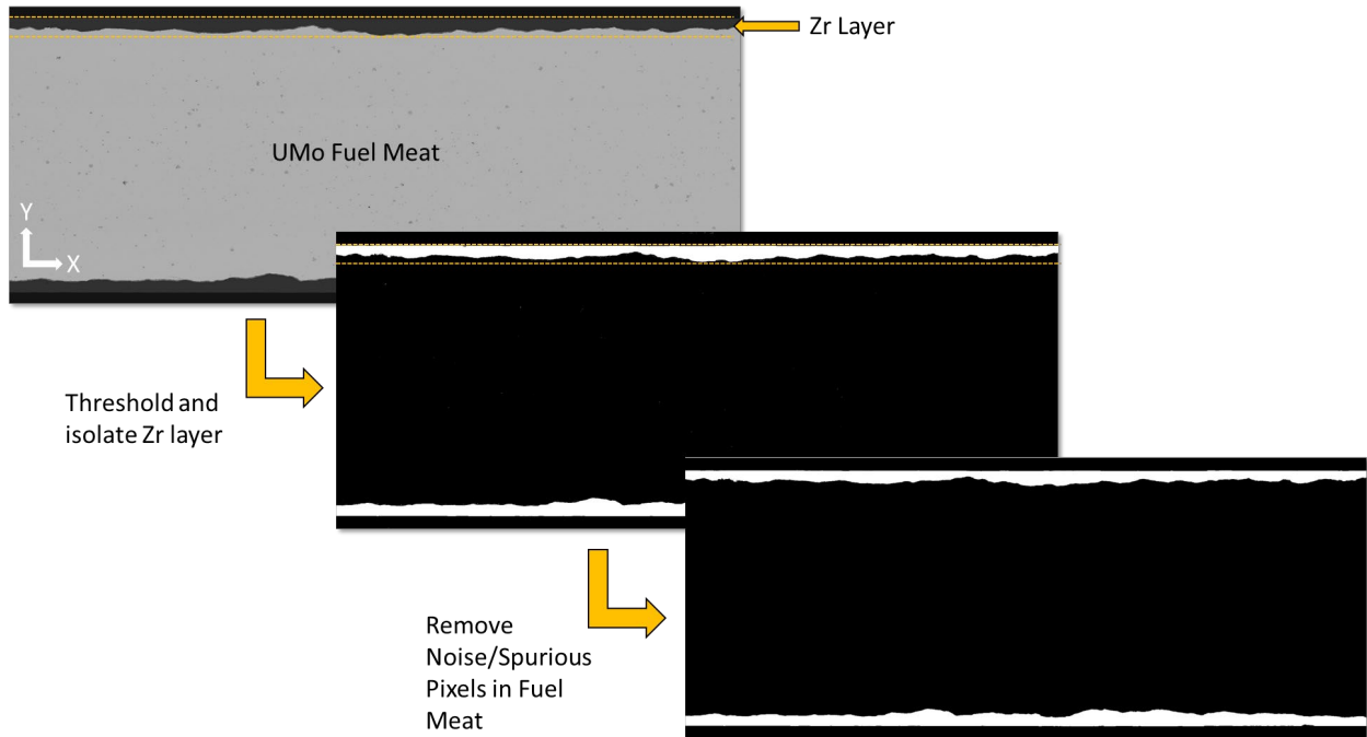
Figure 3. Walk-through visualization of the thresholding process associated with isolating the Zr layer
