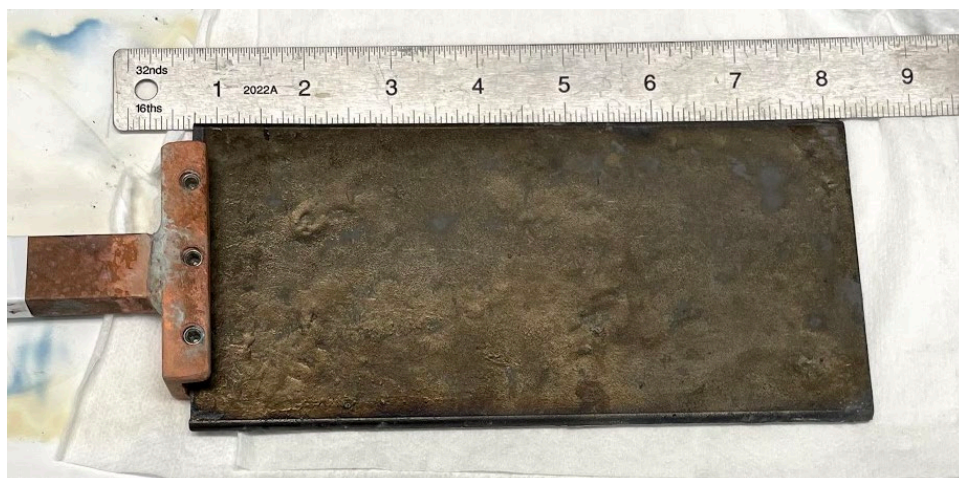
Figure 3. DU-10Mo cast plate with hot top removed and attached to working electrode connection prior to electropolishing
