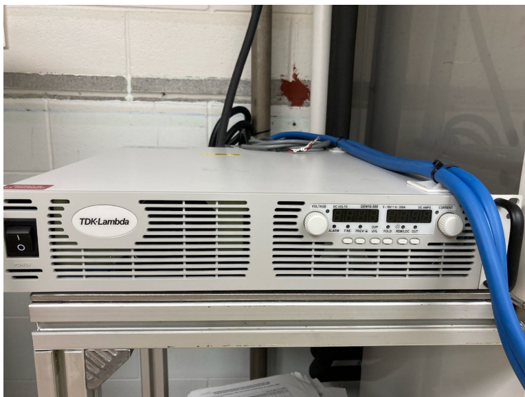
Figure 9. TDK-Lambda Gen 10-500 DC Power Supply used for Electropolishing
