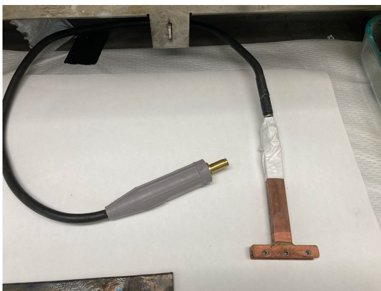
Figure 10. Fabricated Anode Work Piece Connection
