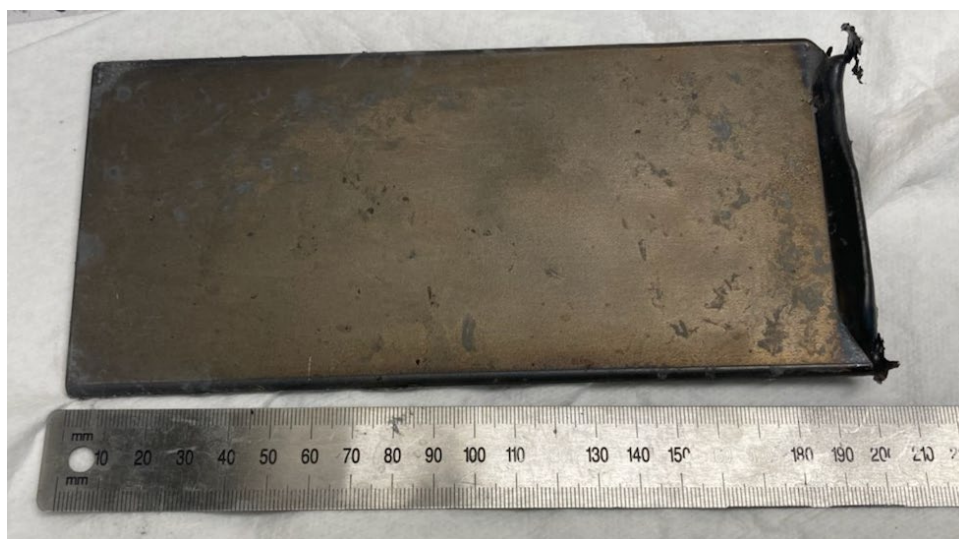
Figure 2. DU-10Mo cast plate with hot top present
