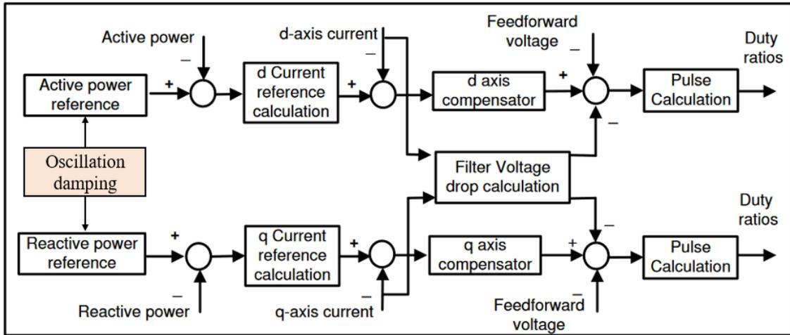
Figure 4-3. Notional IBR oscillation damping control architecture
