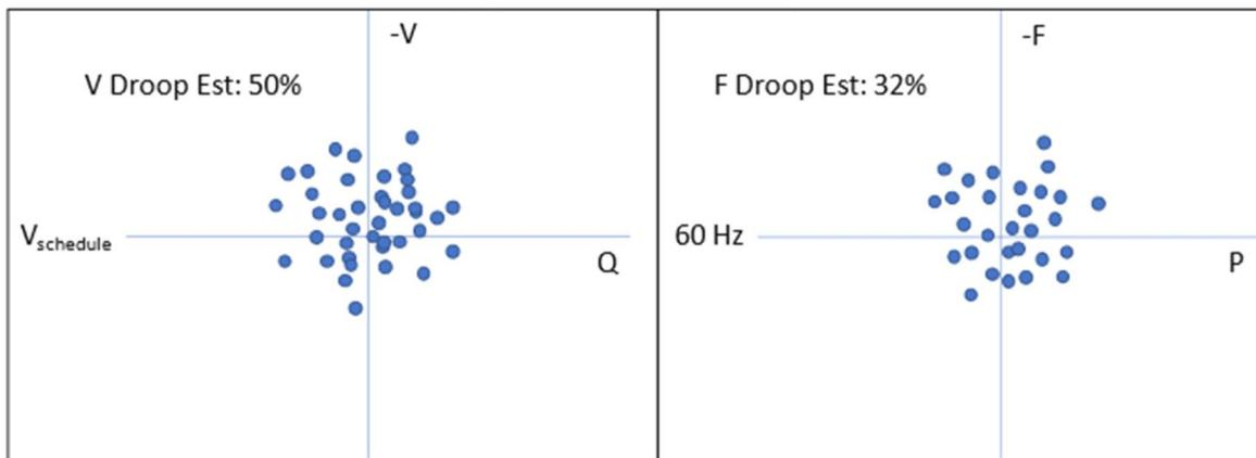
**Figure 2-2. Conceptual illustration of the Generator Scorecard report for two generators. These diagrams are based on images shared by BPA.**
