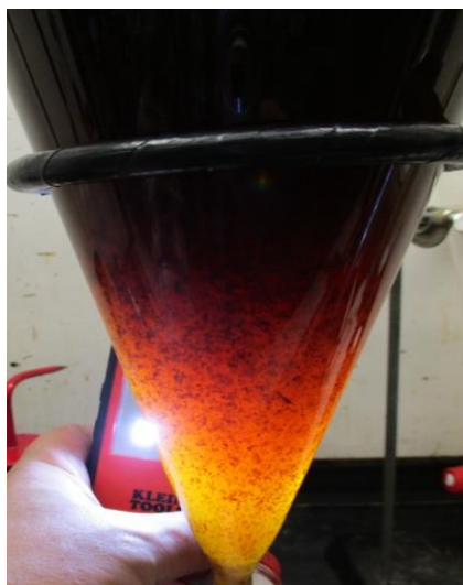
Figure 2. Biocrude-water separation during HTL processing of Picochlorum celeri .
