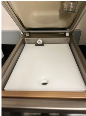
Figure 10. Inserted Filler Plates in Chamber
