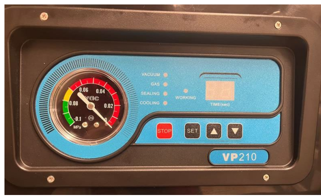
Figure 13. Vacuum Chamber Control Panel
