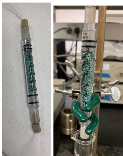
Figure 2. Photograph of MOF-polymer granules (engineered form) packed column for stability test
