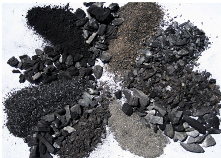
Figure 3. A diverse collection of biochars made from different feedstocks by a variety of production methods (University of California-Davis Biochar Database; http://biochar.ucdavis.edu/ ).
