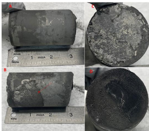
Figure 2: VC-1 billet before cleaning. A) The billet side view. B) The opposite side view with an arrow indicating where the crucible and melt reacted. C) The billet bottom contacting the crucible bottom. D) The billet top which was exposed to the VIM environment.
