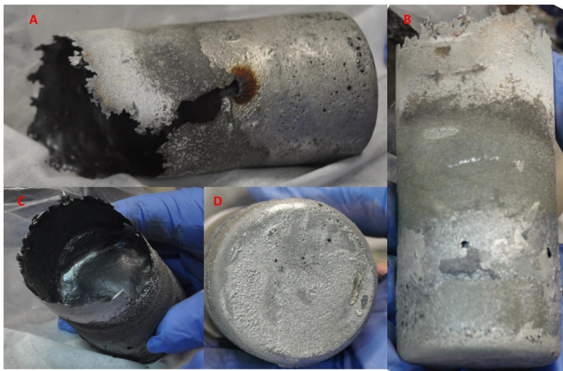
Figure 6: VC-2 billet before cleaning. A) billet side view. Just below (to the right) of where the brown halo is seen is the top of the continuous billet. Above that (to the left) of the halo is a very thin layer that was adhered to the crucible walls but not part of the continuous billet. B) The opposite side view of the billet. C) Top view of the billet which was exposed to the VIM atmosphere. The thin layer adhered to the crucible can be easily seen extending past the top of the billet. D) The bottom of the billet which was in contact with the \text{ZrO}_2 crucible
