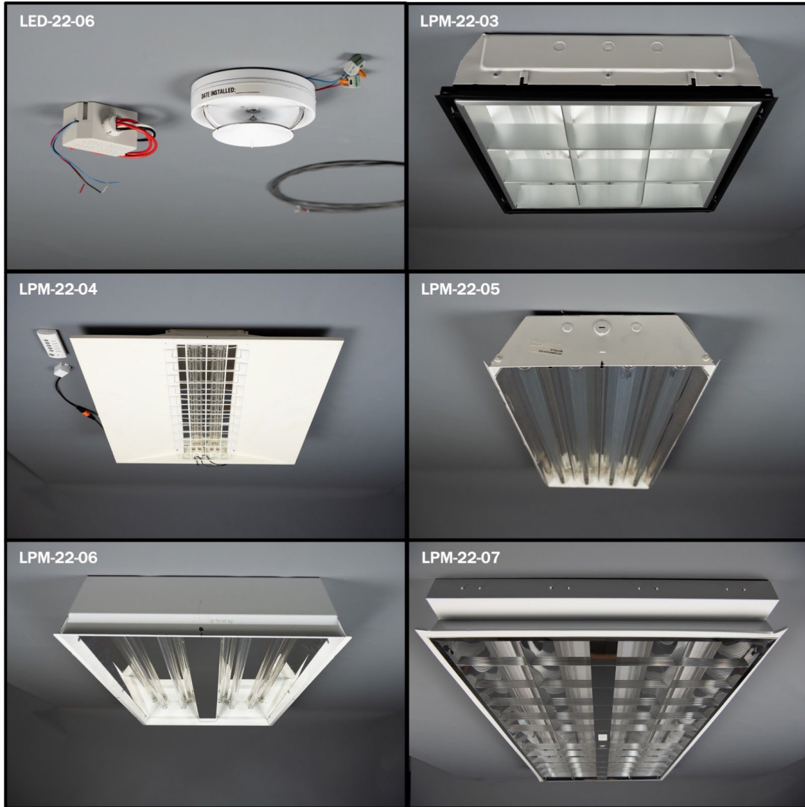
Figure 3. LED and LPM whole-room luminaires, viewed from below and to one side. LED-22-06 had a 5-inch diameter and protruded 2.1 inches below ceiling. LPM-22-03 and LPM-22-04 were 2x2 troffers, measuring 2 feet on each side in plan. LPM-22-05 was a high-bay luminaire measuring 14x48 inches in plan. LPM-22-06 and LPM-22-07 were 2x4 troffers. Troffers are intended to be recessed into the ceiling but are shown surface-mounted. Photo credit: PNNL (Andrea Starr).
