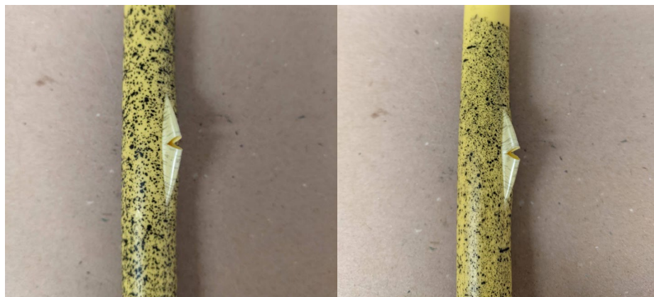
Figure 19. MDPE burst test specimens displaying ductile failure; (left) hydrogen exposed specimen; (right) control specimen not exposed to hydrogen 43
