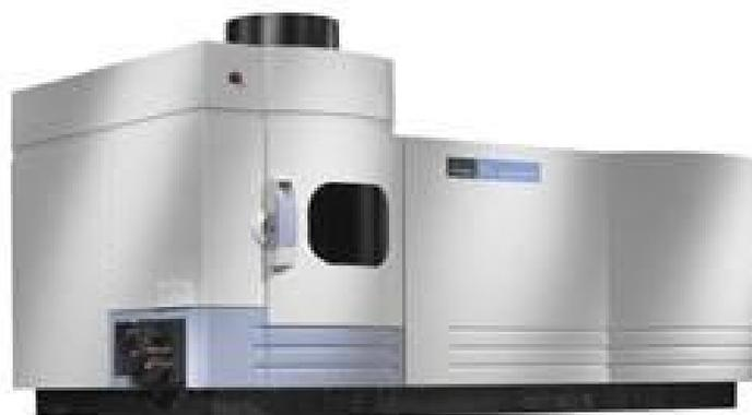
Figure 4: Optima 5300 ICP-OES
